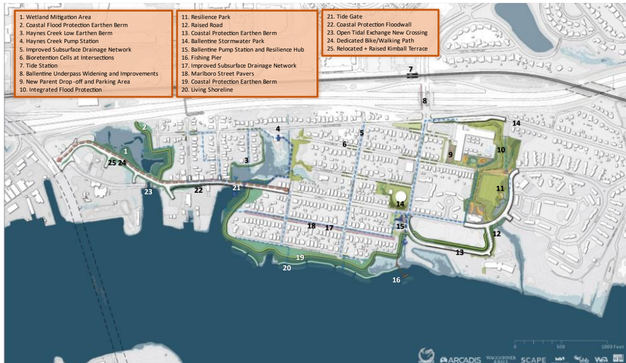
Figure 1. Components of the Ohio Creek project that contributed to flood risk reduction, coastal protection, and recreation measures implemented. Image courtesy of the City of Norfolk.
