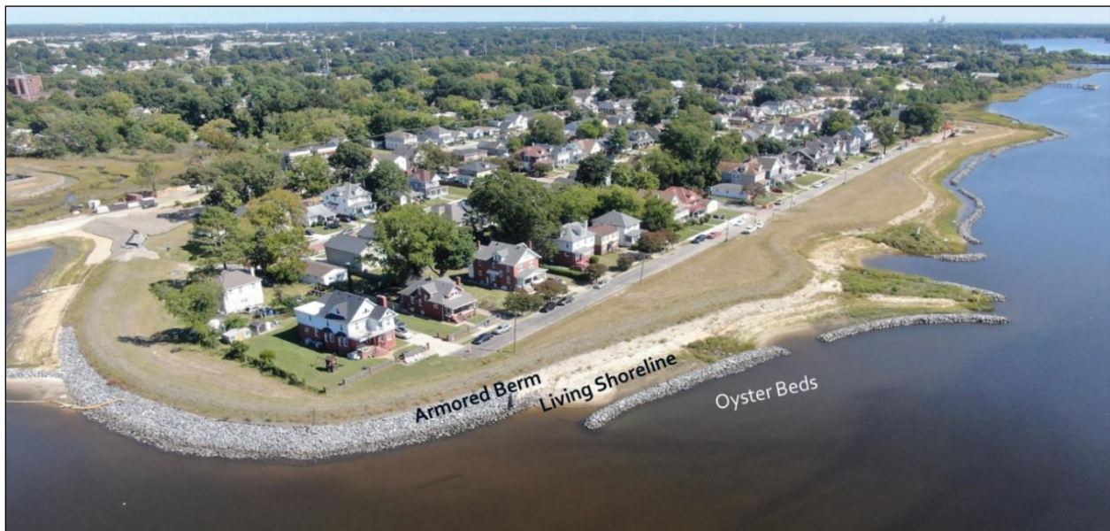
Figure 4. Aerial photo of the coastal measures used to reduce flood risk and shoreline erosion, including an earthen berm (armored riverside), living shoreline, and oyster beds. Image courtesy of the City of Norfolk.
