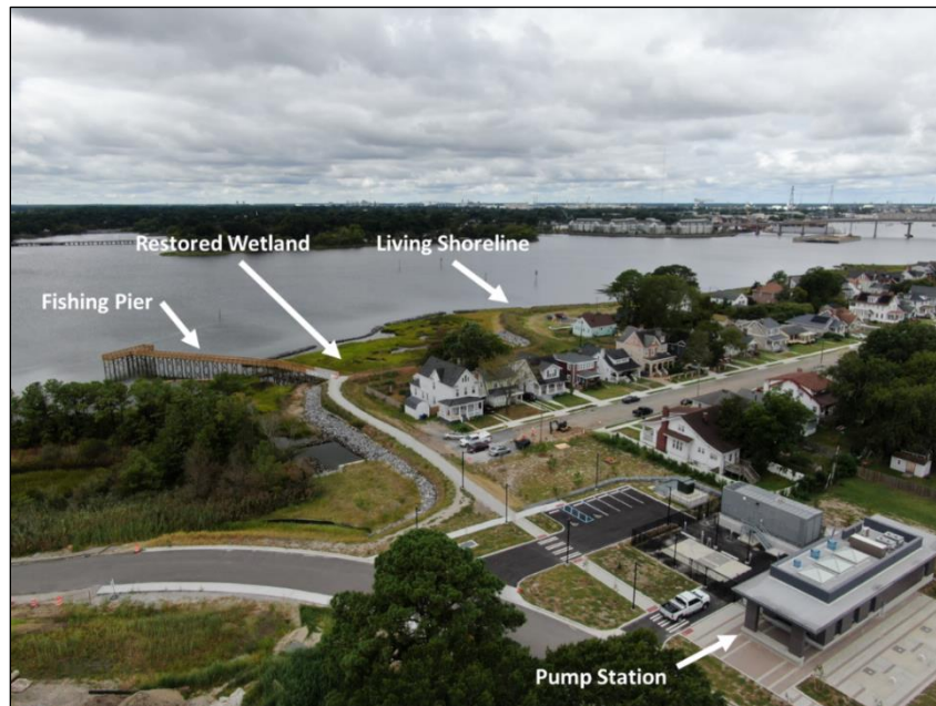
Figure 2. Aerial view of a section of the completed Ohio Creek flood risk management project. Notable project features shown include the fishing pier ( middle left ), restored wetland (immediately to the right of the pier), pump station ( lower right ), and living shoreline ( middle center and right ) along the right descending bank of the Elizabeth River. Image courtesy of the City of Norfolk.
