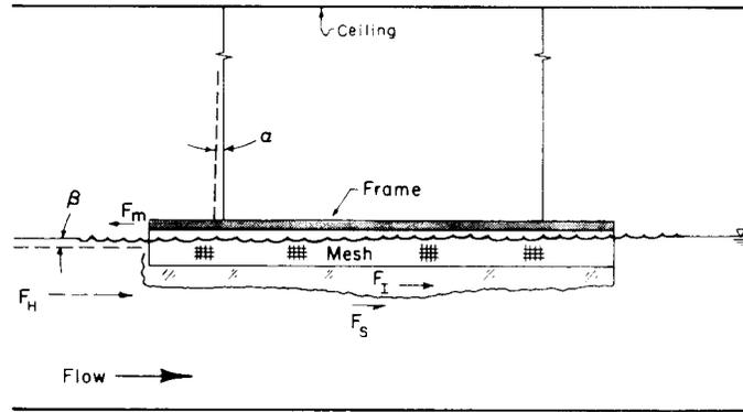
Figure 1. Experimental setup in flume.
