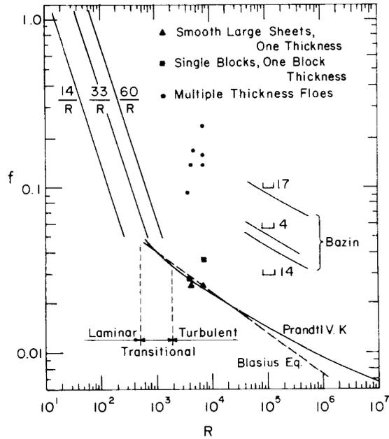
Figure 10. The friction factor-Reynolds number relationship for open channels with different flow regimes (see Chow 1959).
