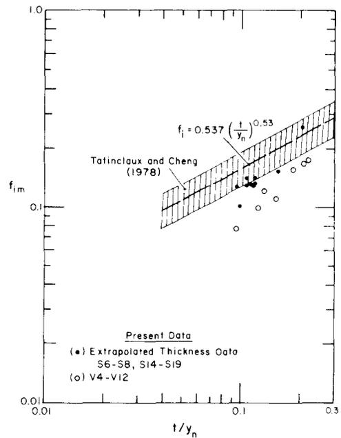
Figure 9. Relationship between Darcy's  $f$  and the normalized ice cover thickness compared with Tatinclaux and Cheng's 1978 data points which are represented by a shaded area containing 90% of their data.
