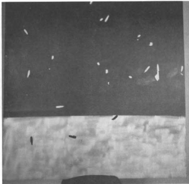
Figure 15. .50 caliber (12.7-mm) machine gun target. Fifty rounds were fired at snow trench from 50 ft.
