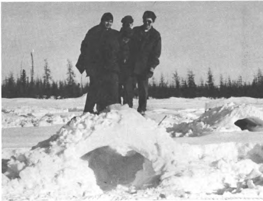
Figure 28. Snow arch after age hardening.
