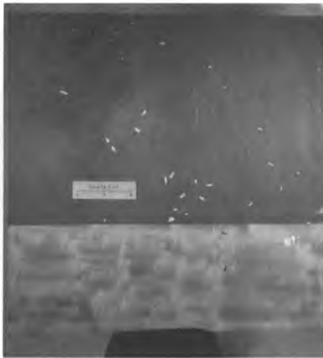
Figure 13. M60 (7.62-mm) target. Fifty rounds were fired at snow trench from 15 m.
