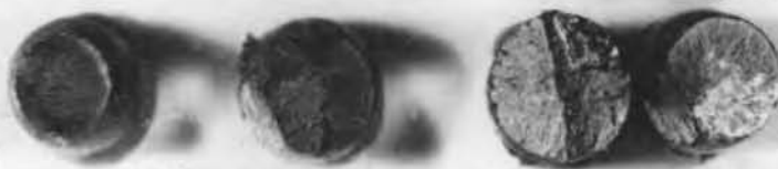
Figure 10. Failure surfaces of some rebars. A 1-cm scale is shown.
