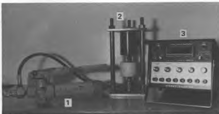
Figure 1. Axial double point-load system. From left to right: (1) hydraulic pump, (2) test frame with load cell (top), hydraulic ram (bottom) and test sample (center), (3) digital strain indicator.
