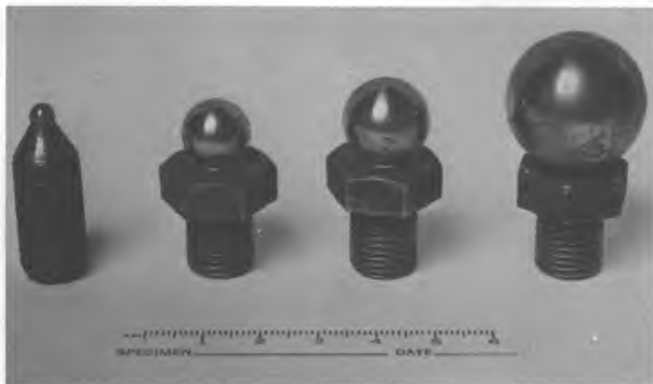
Figure 5. Configuration of the four ball points used in the axial double point-load tests.
