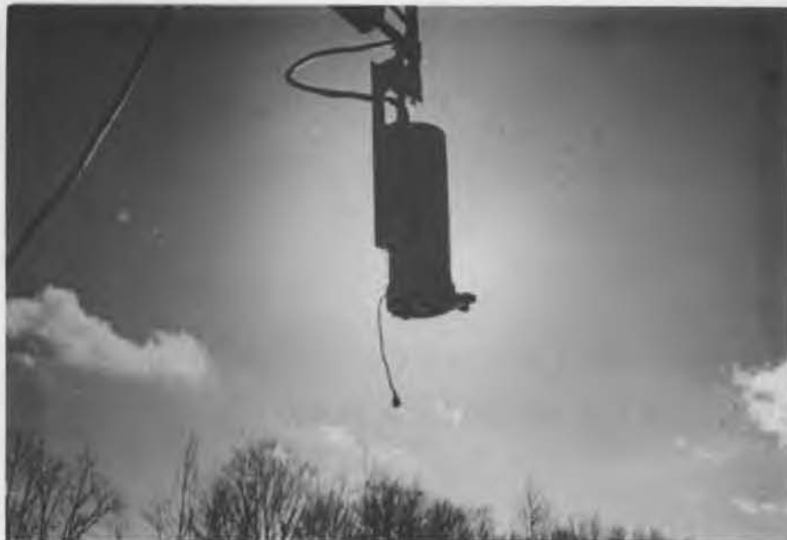
Figure 1. Radiometer head suspended from boom, looking vertically downward.
