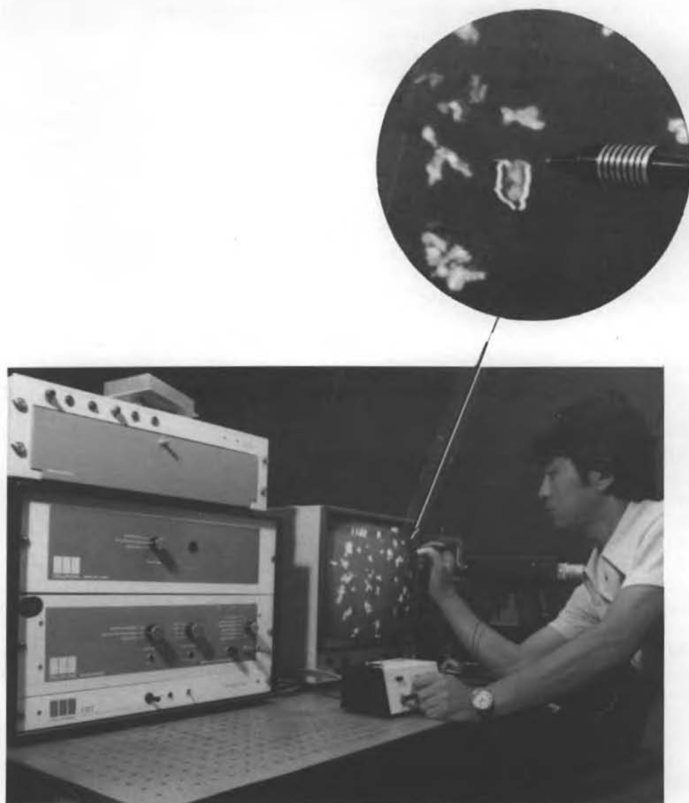
Figure 2. Particle measurement computer ( \mu MC) used in size analysis of some replicas of snow grains.
