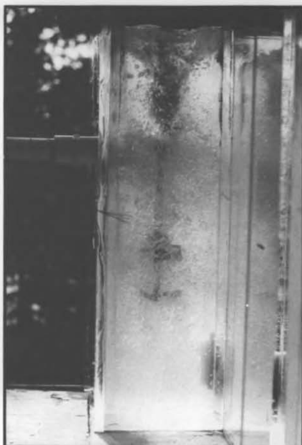
b. Turbulence in rapid mixing unit.
