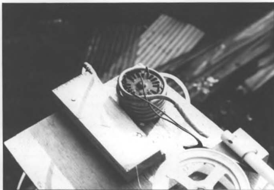
c. Cooling coil on rapid mixing unit.
