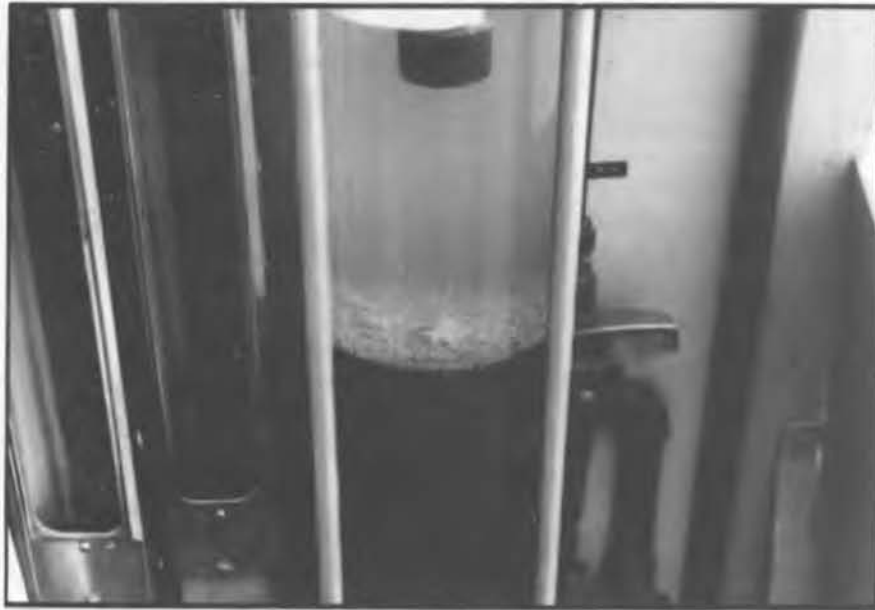
Figure 14. Pinfloc formation suitable for direct filtration.
