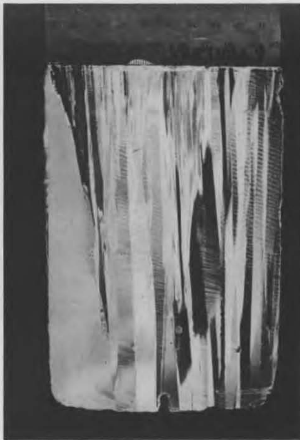
Figure 14. Vertical thin section from fresh water ice block (scale in cm).
