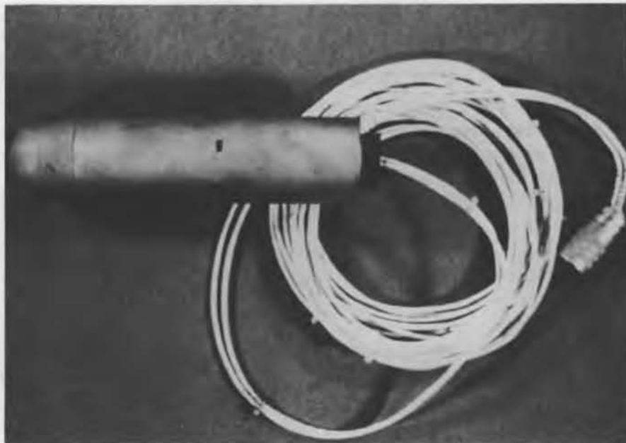
Figure 1. Biaxial ice stress sensor.
