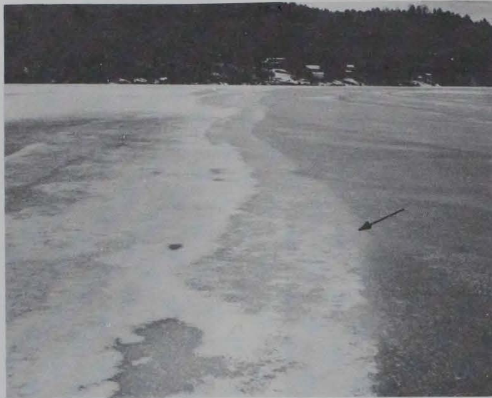
Figure 6. Ice-growth boundary of the kind shown in Figure 5b. The ice on either side of the boundary formed approximately four days apart.
