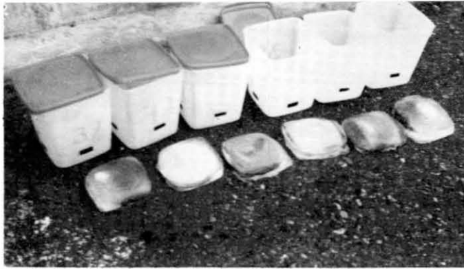
Figure 2. Preparation of UAG samples. The six identical plastic containers are shown with the six samples that were prepared. The black markers on the containers indicate depth of filling. The six substrates – aluminum, steel, brass, asphalt, concrete, and porous stone – are frozen into the bottom of the samples.
