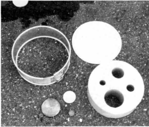
a. Separate components – mold, substrates, and gasket assembly. The fourth hole in the mold was intended to provide unobstructed passage of the optical beam when the mold with samples was inserted into the optical system. Removal of the samples proved to be more feasible so this feature was never used.
