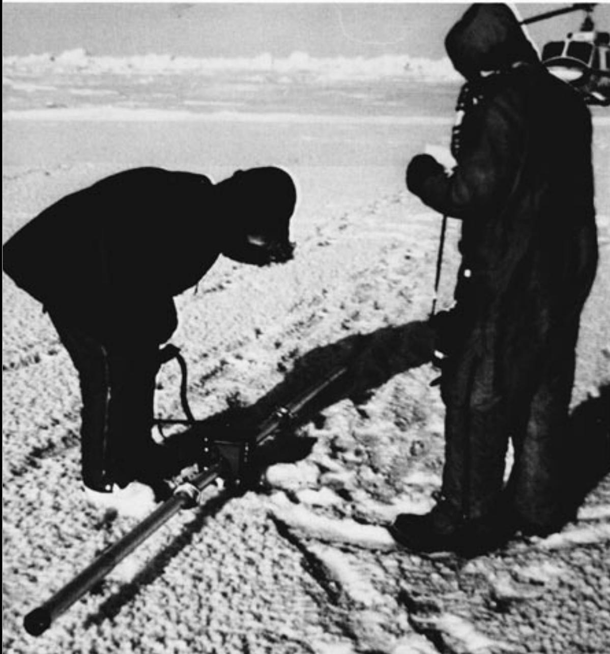
**Abstract:** Field results from a man-portable electro-magnetic induction sounding instrument, with special plug-in data processing modules for the remote measurement of sea ice thickness, are discussed. The field trials indicate that the instrument was capable of estimating undeformed sea ice thickness, with a snow cover, generally within about 5% of the drill hole
