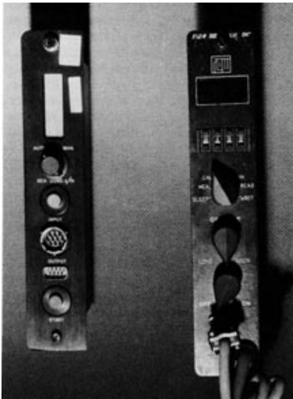
Figure 3. The Geonics (left) and Flow Research ice thickness modules.
