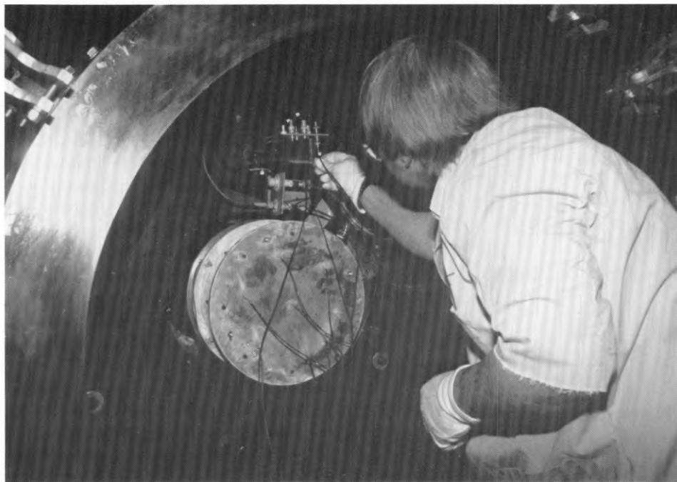
Figure 9. Snow target mounted in the gas gun target chamber.
