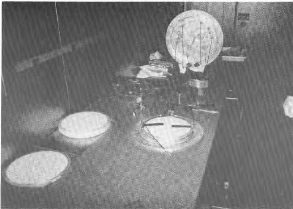
c. Snow wafers and gauges installed at an intermediate stage of target construction.
