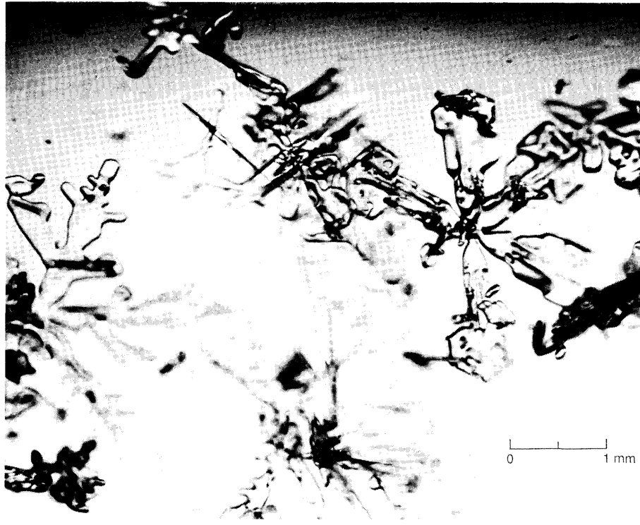
Figure 18. Snow grains from metamorphic layer 1. Partial and nearly complete dendrites and spatial dendrites are present. Crystal edges are smooth and rounded, suggesting that vapor transfer is taking place.
