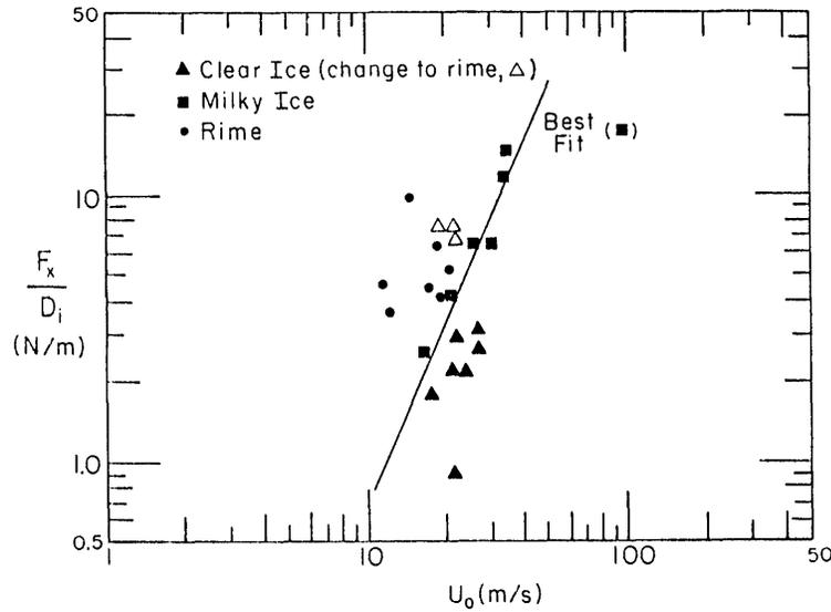
Figure 4. Horizontal force  $F_x$  normalized to the accretion diameter  $D_i$  vs the wind speed normal to the wire for rime ice, milky ice and clear ice accretions. The best-fit line for the milky ice accretion is shown. (After Govoni and Ackley 1983.)
