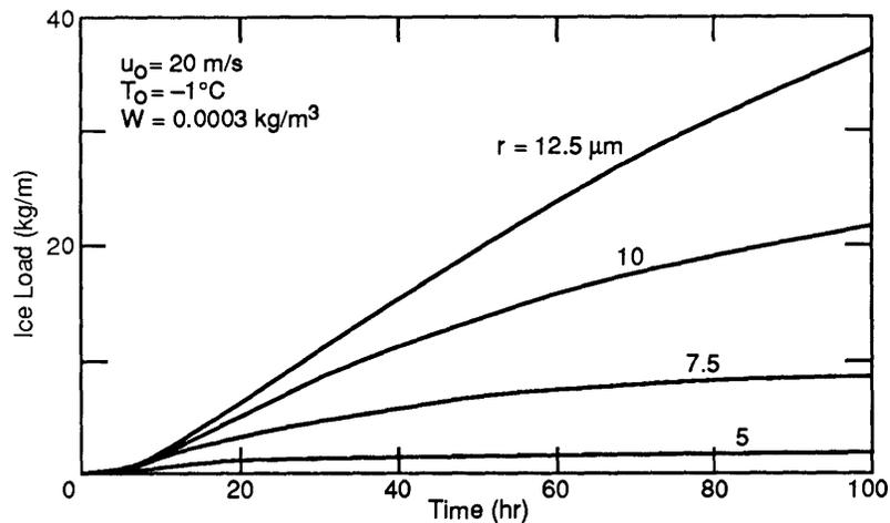
Figure 1. Dependence of accreted ice load on the median volume droplet diameter. (After Makkonen 1984b.)
