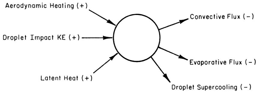
Figure 3. Heat balance at the freezing surface. (From Ackley and Templeton 1979.)
