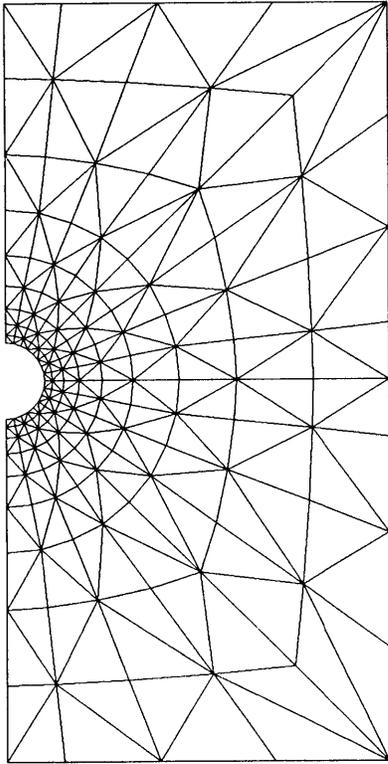
Figure 6. Finite-element mesh for the wire icing program.
