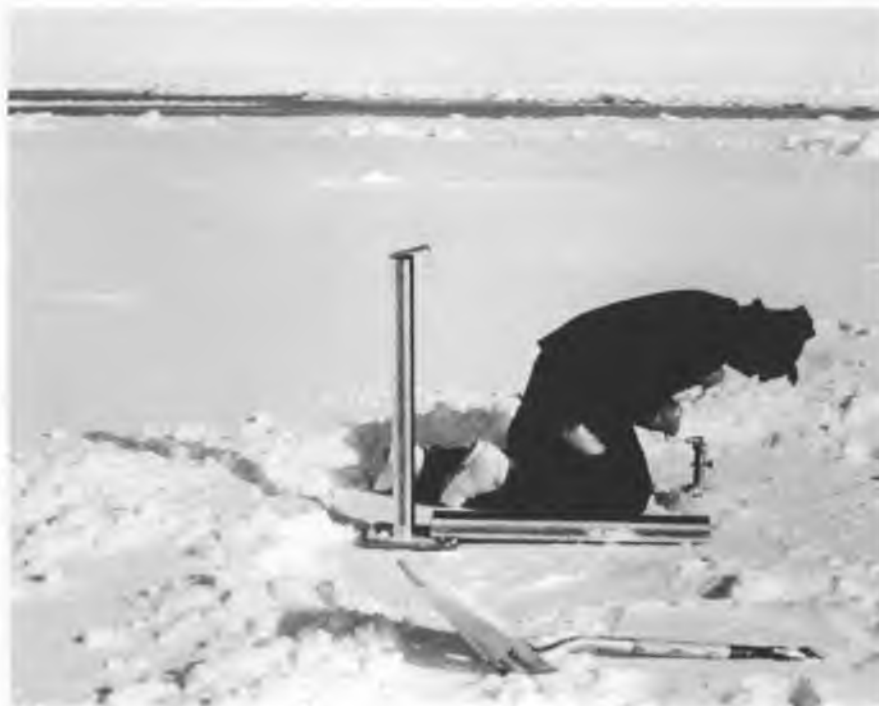
Figure 5. Coring a multi-year floe. Also shown is the insulated split-tube core sampler used for measuring ice temperatures and for cutting cores for salinity measurements.
