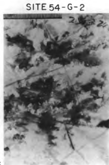
Figure 14. Vertical thick sections showing wafer-like and plate-like crystals of ice in deeper parts of floes 54-A-1 and 54-G-2, respectively.
