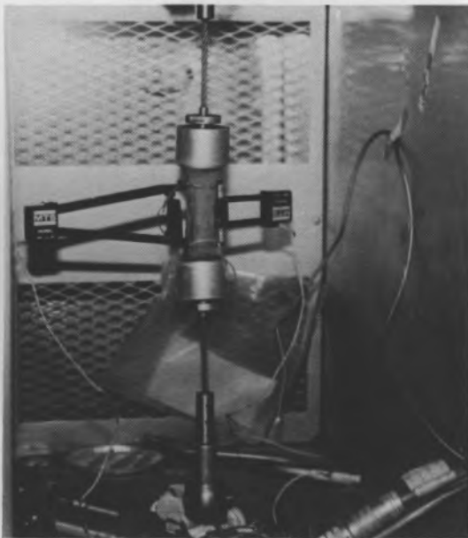
Figure 7. A specimen bonded with two extensometers ready for testing.
