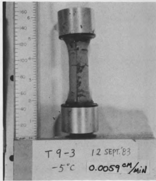
b. \theta = -5^{\circ}C , \dot{\epsilon} = 1.2 \times 10^{-5}/s , \gamma_d = 1.355 g/cm^3 .
