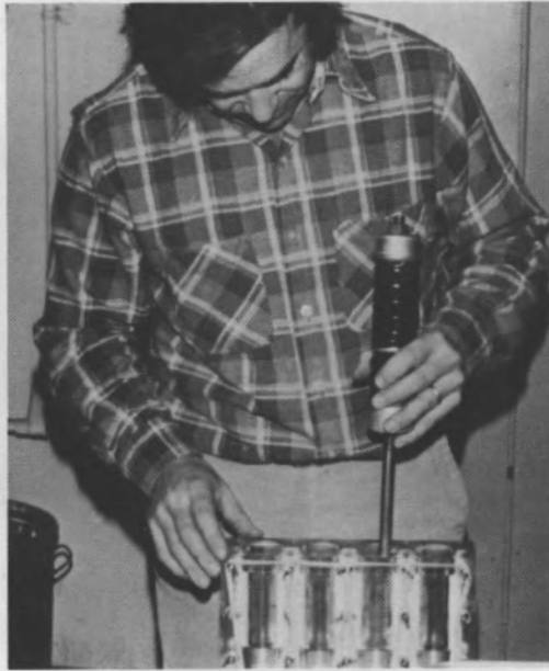
Figure 1. Compacting specimens in the Lucite gang mold.
