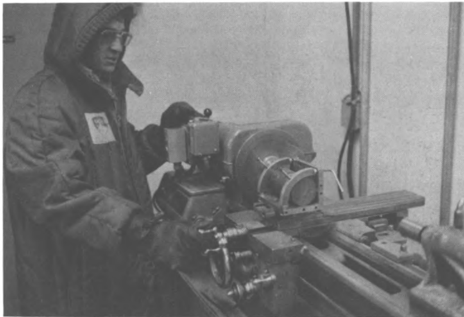
Figure 6. Trimming a specimen on a lathe in a coldroom.
