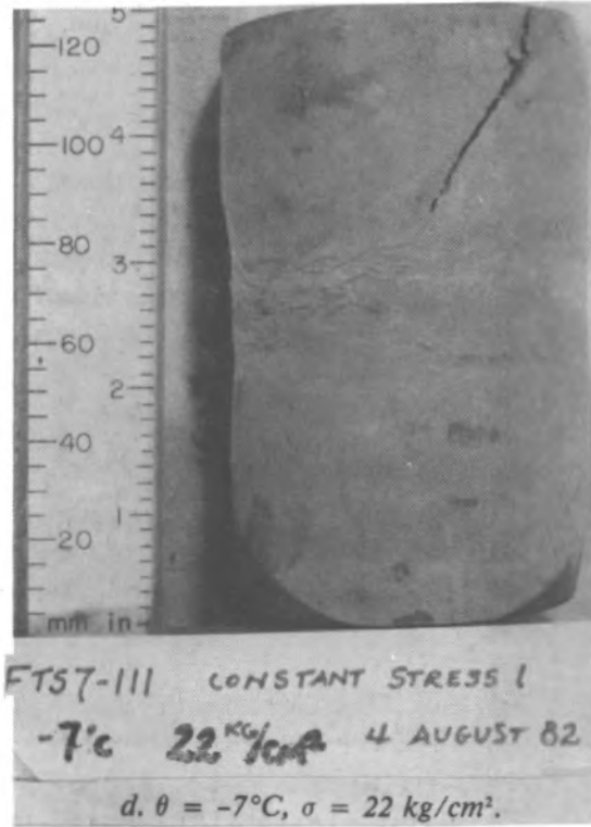
Figure 19. Typical Fairbanks silt specimens after long-term creep tests, showing X-shaped shear cracks.
