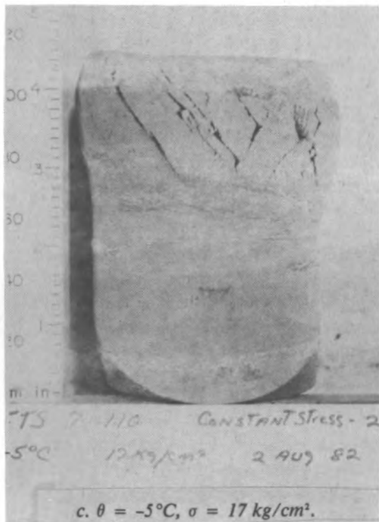
Figure 19. Typical Fairbanks silt specimens after long-term creep tests, showing X-shaped shear cracks.
