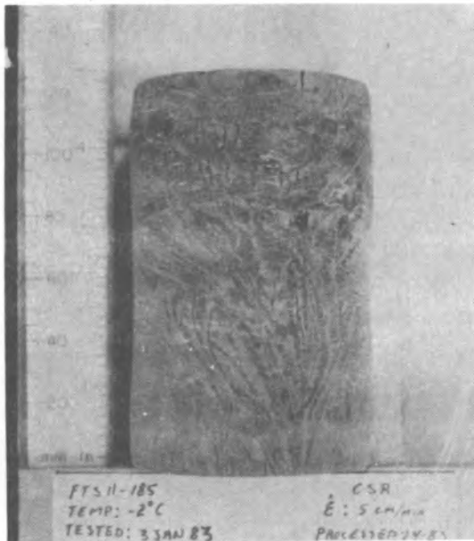
a. Cracks in a low-density sample.
