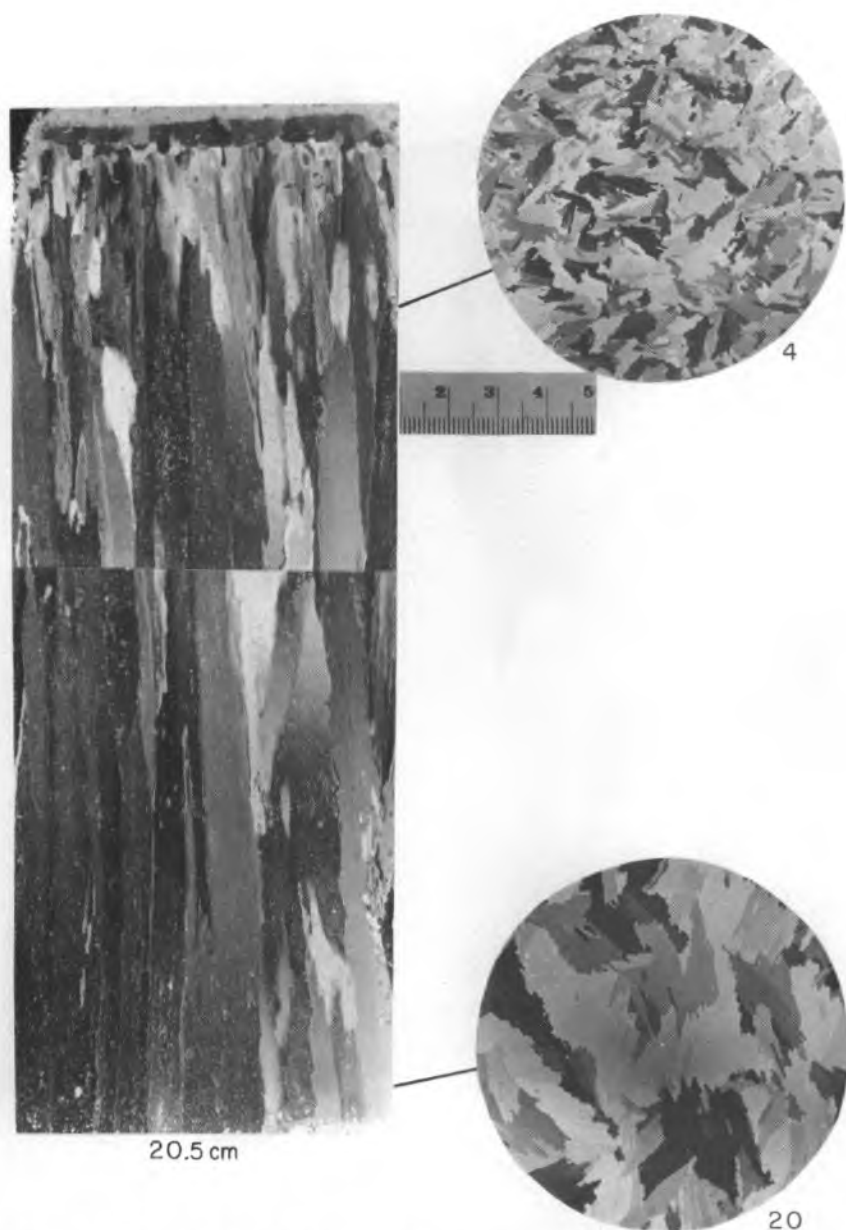
Figure 4. Vertical and horizontal thin sections of structure of ice sheet from which slabs 84-3 and 84-4 were obtained. Scale subdivisions on photographs are 1 mm.
