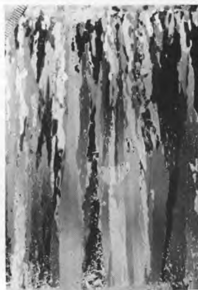
Figure 15. Vertical and horizontal thin sections of structure of ice in slab 85-3 after testing and thermal modification. Smallest scale subdivisions are 1 mm.
