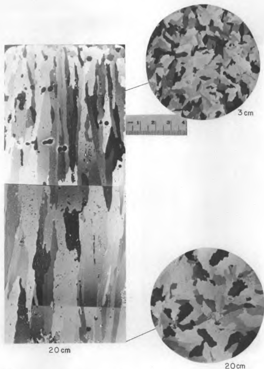
Figure 5. Vertical and horizontal thin section structure in thermally modified ice slab 84-3. Scale subdivisions are 1 mm.
