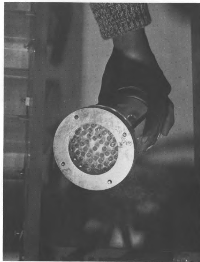
d. Bottom view of test cylinder with solution exit holes.
