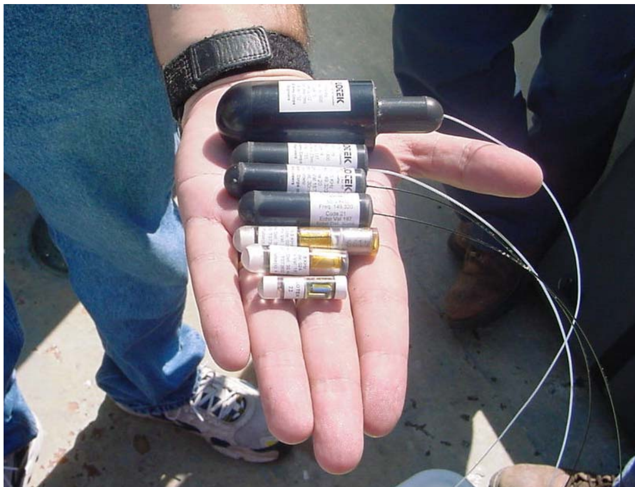
Figure 1. Radio (upper four) and sonic (lower three) tags and their typical size ranges (manufactured by Lotek)
