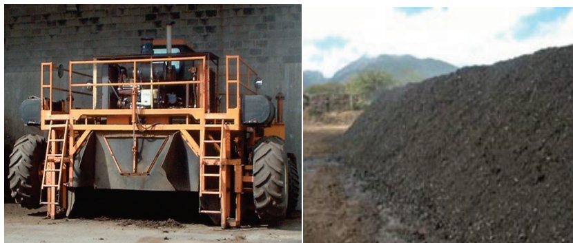
Figure 3. Windrow Composting. Windrow turner and a windrow compost pile.
