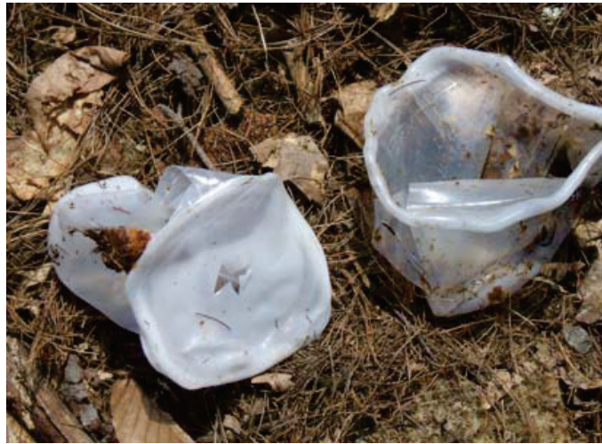
Figure 2. PLA cups partially degraded after 30 days composting [From USCC (2009)].
