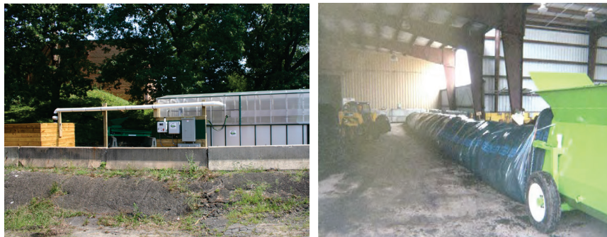
Figure 6. In-vessel compost systems. The system on the left was the enclosed system tested at JBM-HH (described in NDCEE 2013a); to the right is a simple enclosed system using a bag approach.
