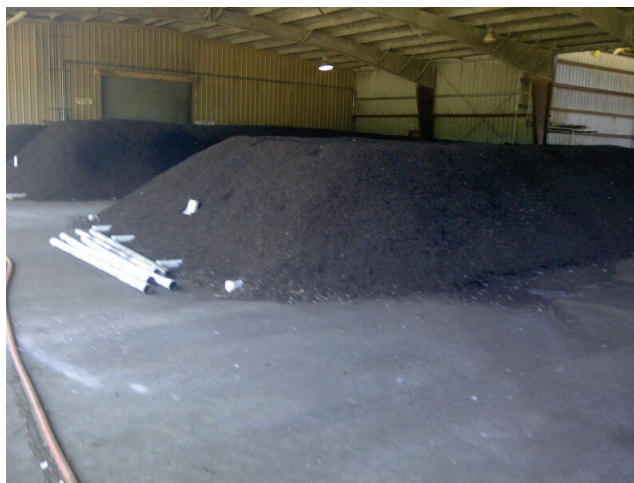
Figure 5. Pictures of JBLM's forced air static pile composting operation.
