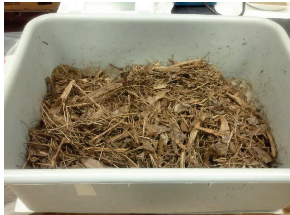
Figure 16. Plastic bin containers used as a compost reactor.
