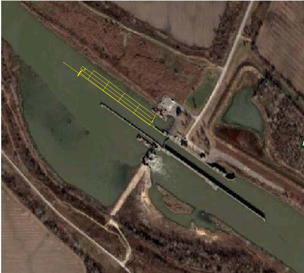
Figure 2.21. Depiction of geometry limited approach angle for 3 x 4 barge tow impacting the guide wall.
