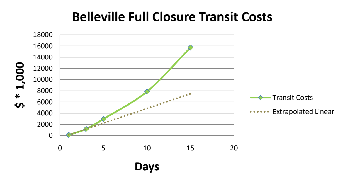
Figure 5.20 The non-linear costs for full closure of the locks and dam at Belleville
