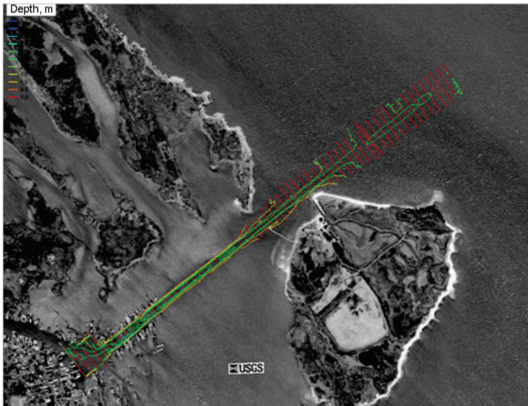
Figure 9. East channel depth contour lines (m, MTL); data locations shown as red points.
