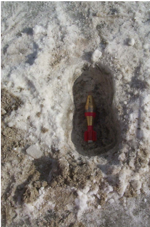
Figure 30. 60-5 placed at ice/sediment interface in 7-in.-thick ice
