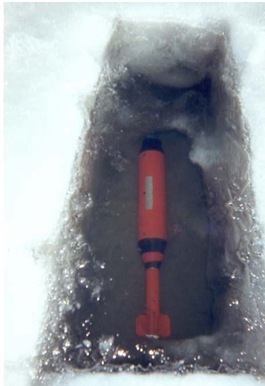
Figure 31. 81H-3 place under 23-in.-thick ice
