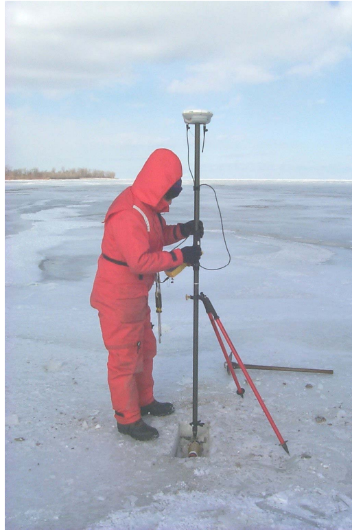
Figure 32. Surveying 81M-5 deployed at ice/sediment interface in 8-in.-thick ice
