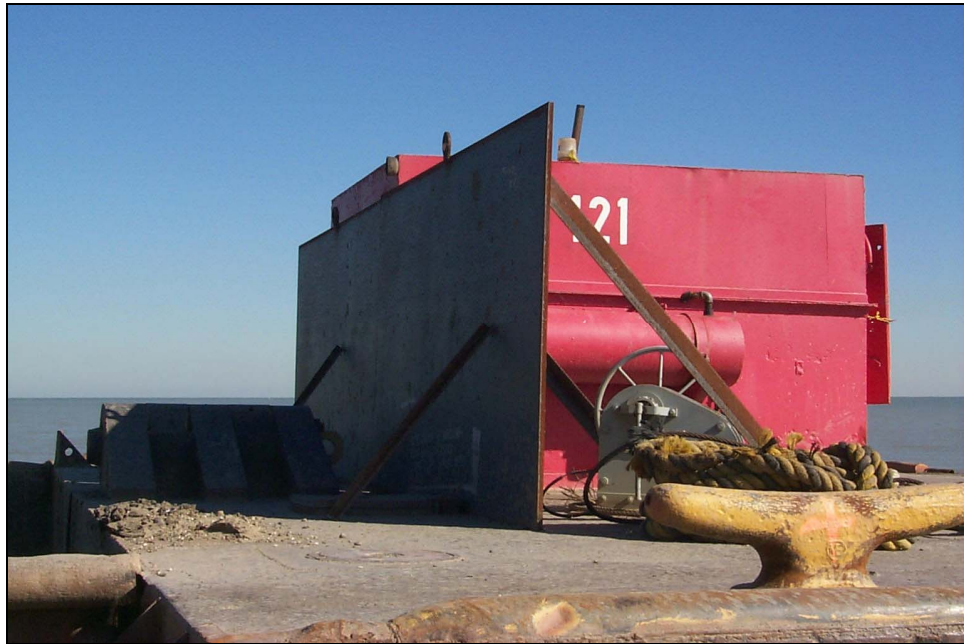
Figure 9. Scow release operators protective barrier
