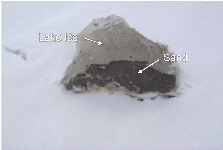
Figure 27. Example of frozen sediment/lake ice interface retrieved during February SO deployment
