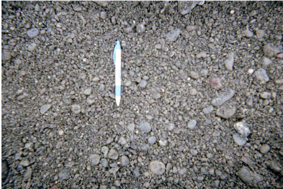
Figure F3. Bed material 1 ft below ground surface, cross section 27 (right side)
