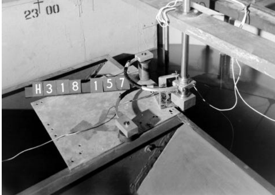
Figure 5. Hawser-pull (force links) measuring device
