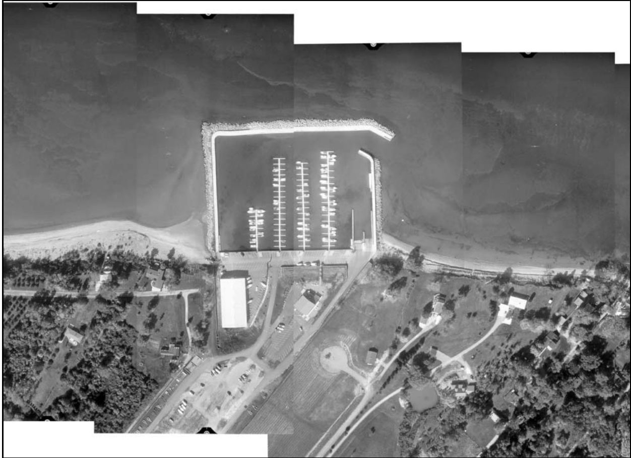
Figure 7. Vertical aerial photograph, October 15, 1999. Shale ledges can be seen through water east (to the right) and lakeward of marina. Bulge in shore west (left) of the marina is accretion on private property that PFBC is unable to mine during biannual bypassing operations
