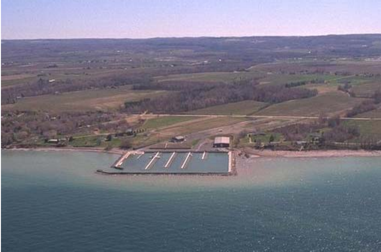
Figure 6. Oblique aerial photograph of marina looking southeast, April 1999. PFBC's spring bypassing operation is in progress, and a backhoe and truck are in the fillet on the right side of the marina. Photograph courtesy Buffalo District
