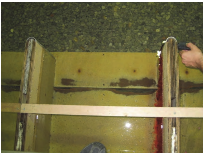
Figure 33. Dye injection at Pump 8 with all pumps operating.
