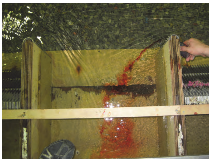
Figure 34. Dye injection at Pump 12 with all pumps operating.
