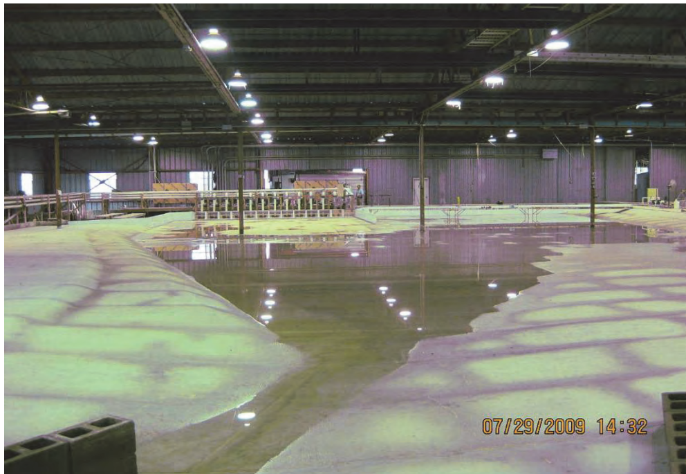
Figure 12. View of original 13-pumps design looking downstream from upstream end of model.
