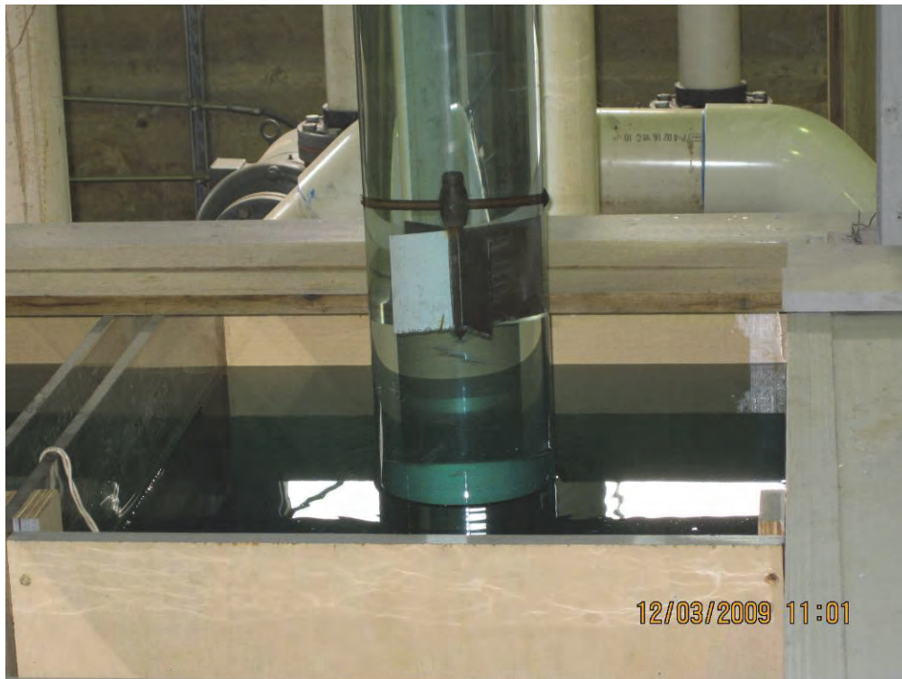
Figure 8. Swirl meter in 6-in. inside diameter acrylic pipe.
