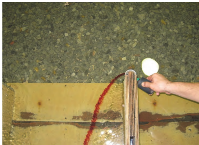
Figure 30. Dye injection for only Pump 8 operating.
