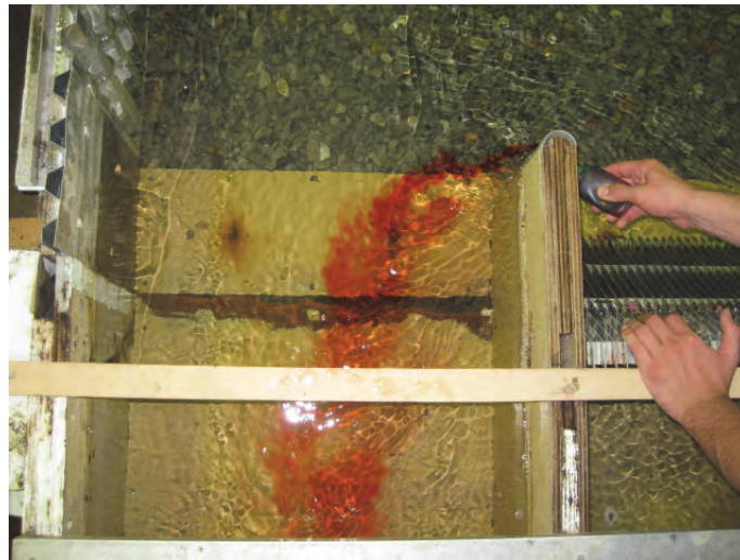
Figure 35. Dye injection at Pump 13 with all pumps operating.
