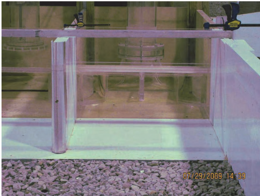
Figure 14. View looking downstream of contracted section and FSI in original design model.
