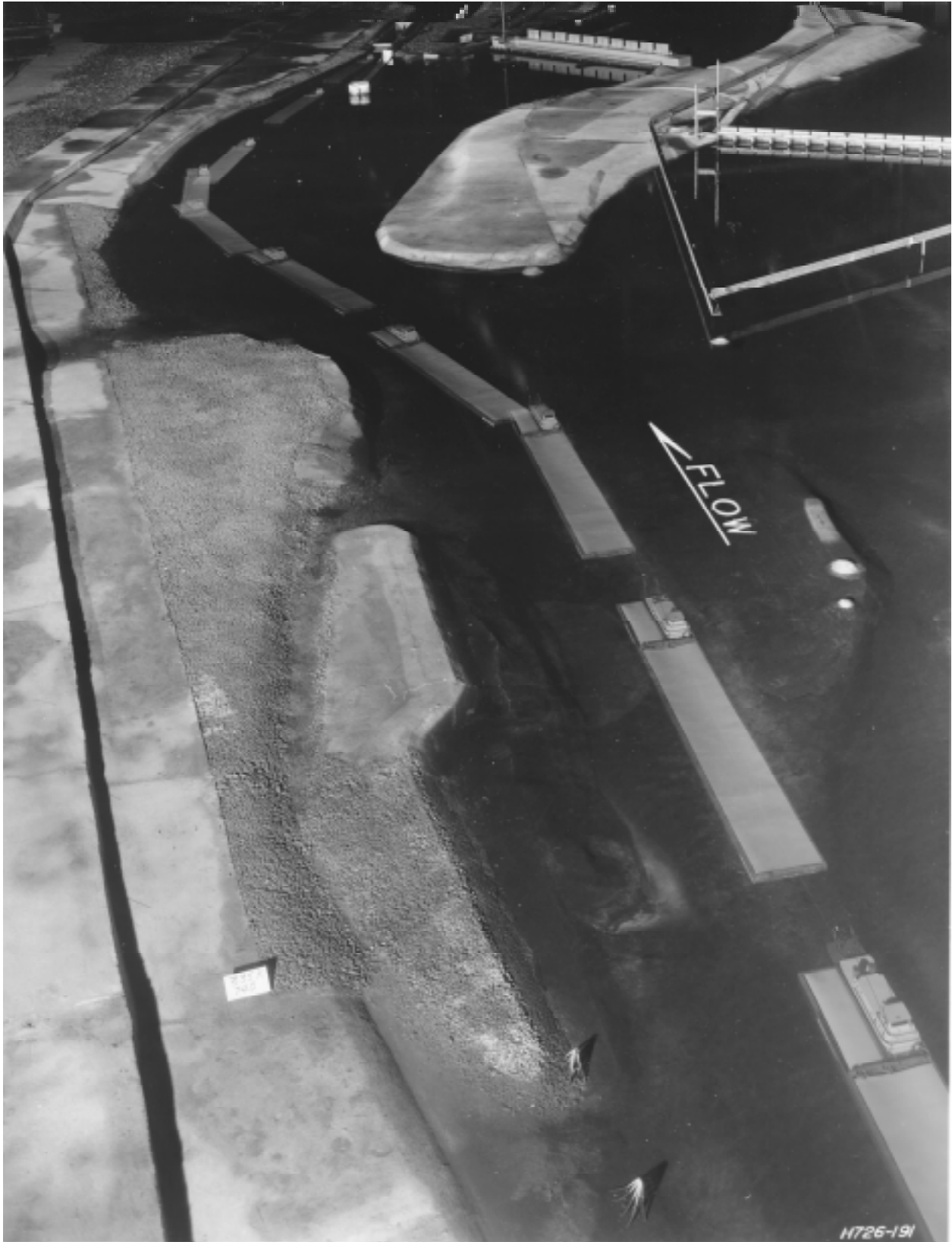
Photo 10. Plan F, 335,000 cfs total riverflow, 140,000 cfs first powerhouse discharge, looking downstream, showing path of upbound tow leaving the new lock
