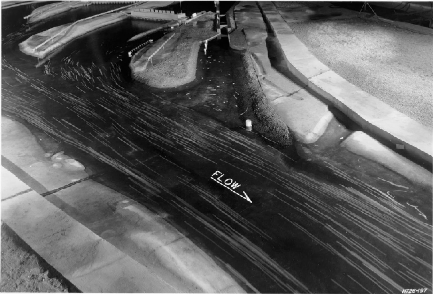
Photo 8. Plan F, looking upstream, 335,000 cfs total riverflow, confetti showing current pattern in vicinity of lock canal
