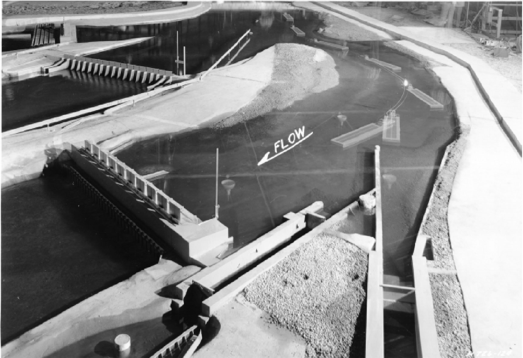
Photo 3. Original design, looking upstream, showing path of downbound tow approaching new lock
