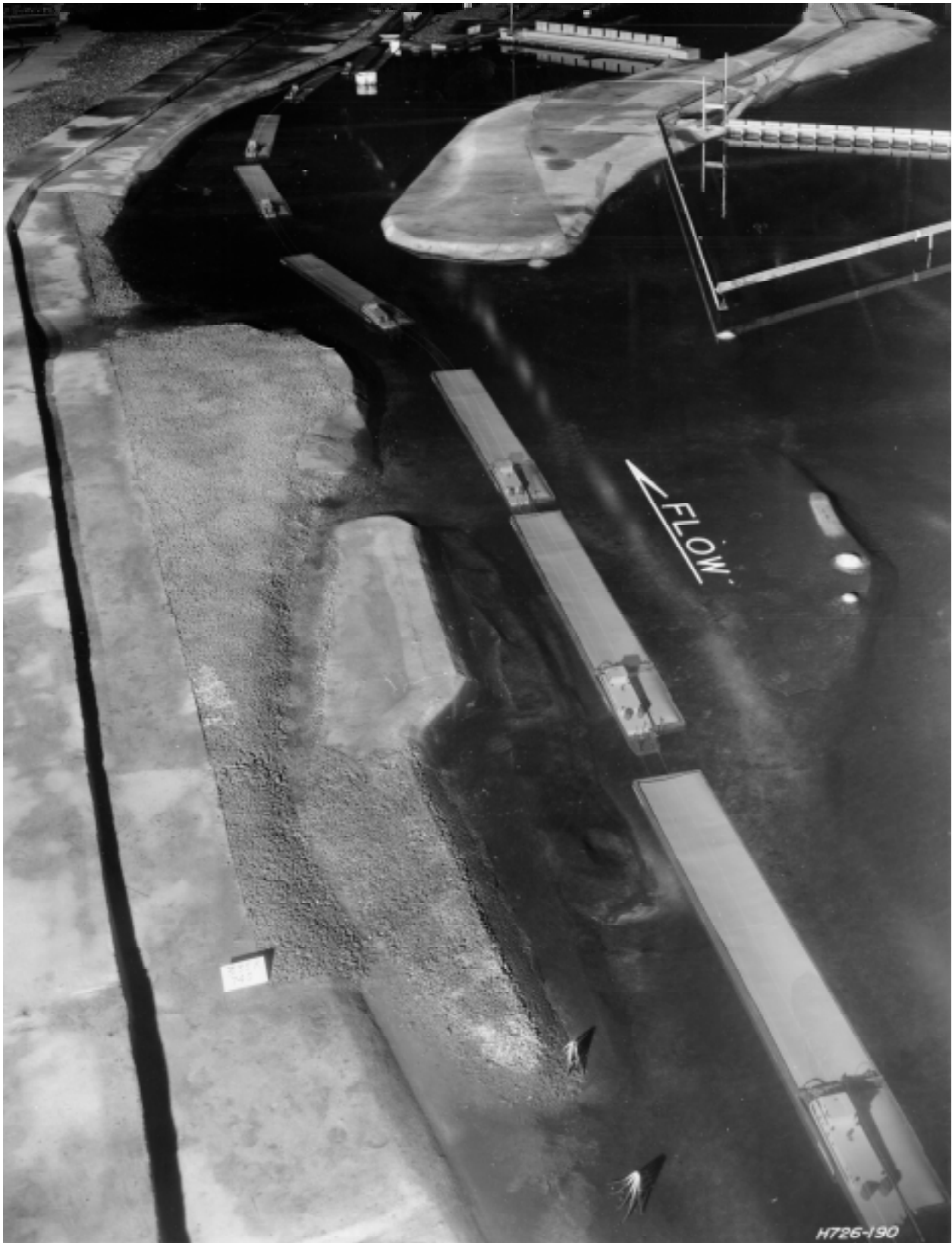
Photo 9. Plan F, 335,000 cfs total riverflow, 140,000 cfs first powerhouse discharge, looking downstream, showing path of downbound tow approaching lock
