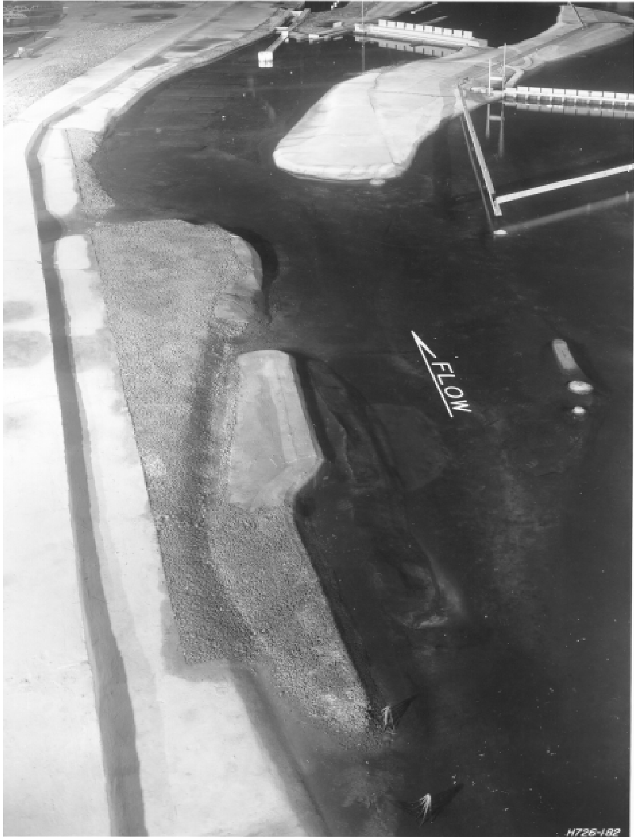
Photo 5. Plan F, looking downstream showing channel alignment
