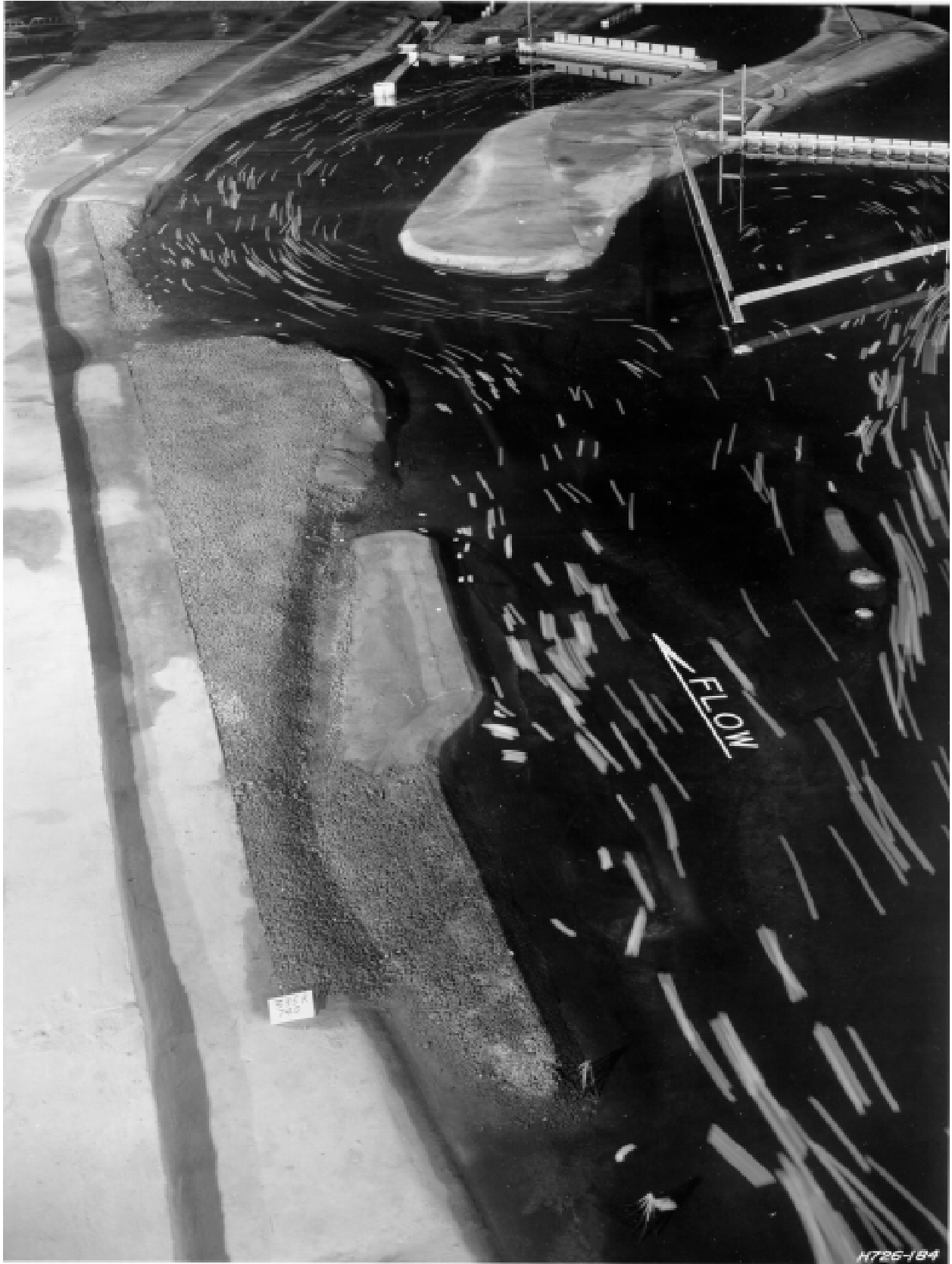
Photo 7. Plan F, 335,000 cfs, looking downstream, confetti showing current pattern
