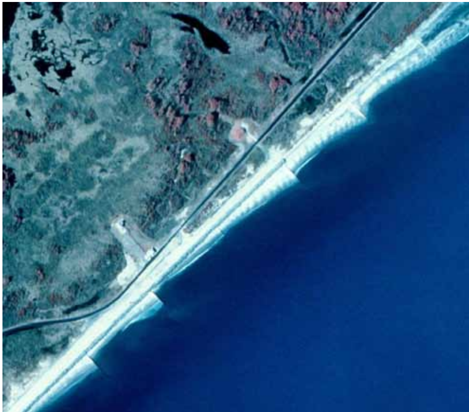
Figure 5-17. Groins field on Wallops Island showing transport direction to the north. Photo taken 20 March 1994.
