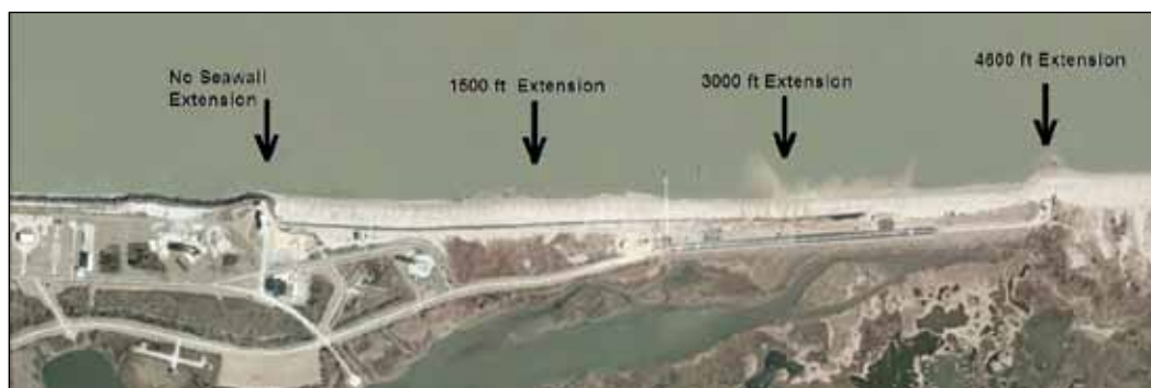
Figure 10-1. Potential seawall extensions modeled in this study.
