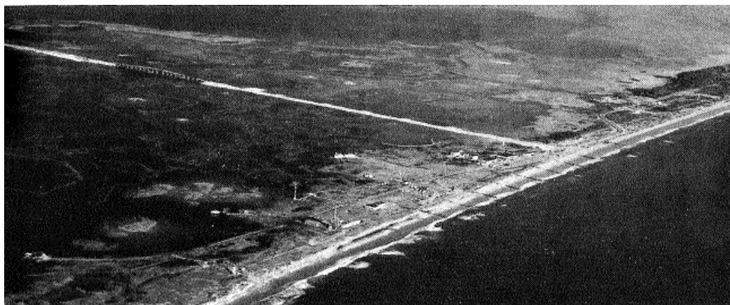
Figure 2-6. Wallops Island, December 1959, showing groin field extending southward from the newly built causeway.
