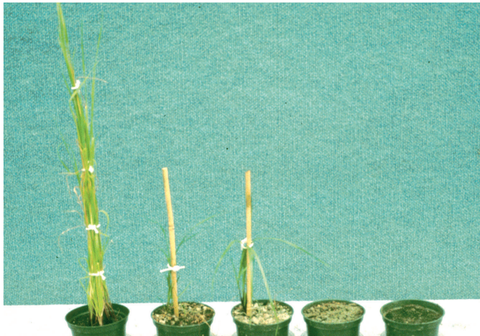
Figure 21. Ryegrass plants growing in blends prepared with dredged material from North Blakeley Site 3 Test 3, at 7 weeks (l to r, Blends 13, 12, 11, 10, and 9)
