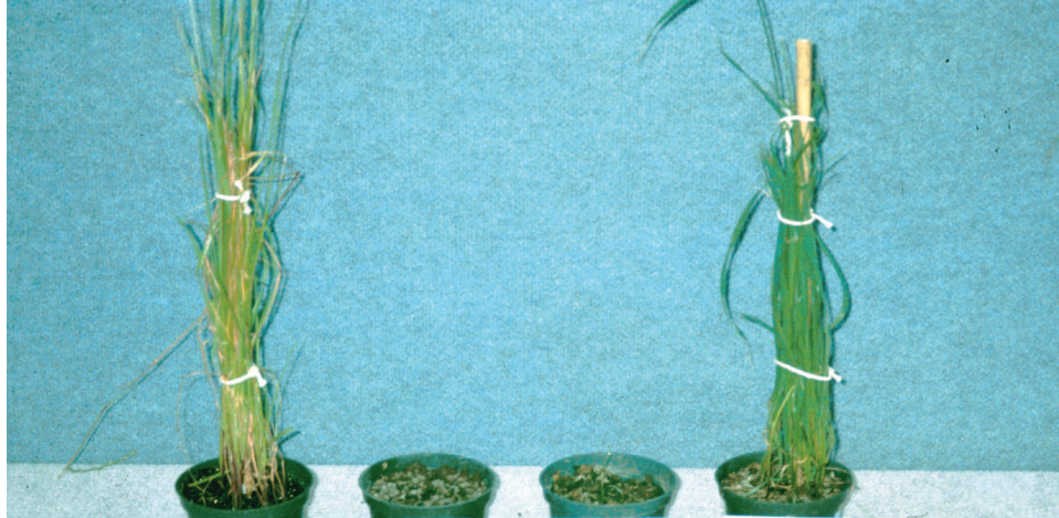
Figure 16. Ryegrass plants growing in Blends 11, 4, 7, and 10 prepared with dredged material from North Blakeley Site 1 and amended with calcium, at 7 weeks (l to r, Blends 11, 4, 7, and 10)
