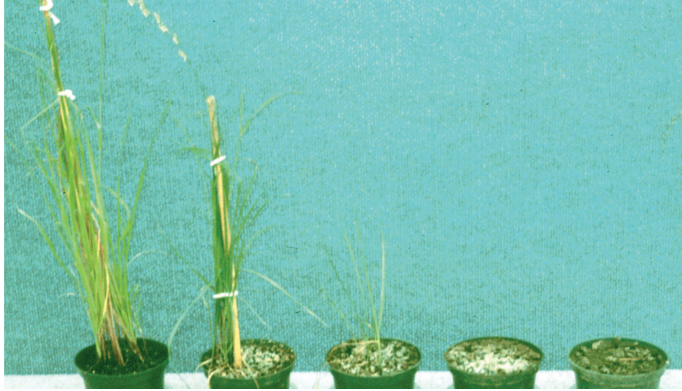
Figure 20. Ryegrass plants growing in blends prepared with dredged material from North Blakeley Site 2 Test 3, at 7 weeks (l to r, Blends 13, 8, 7, 6, and 5)
