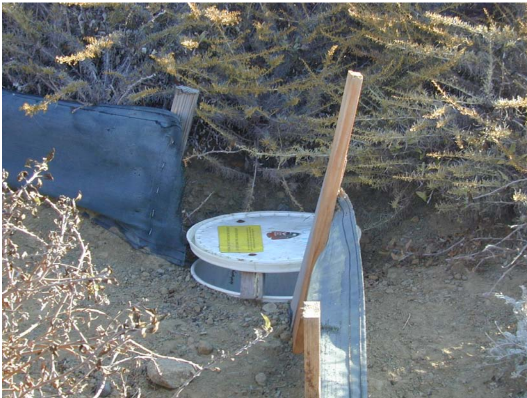
Figure 5. A pitfall trap and associated drift fence station; one of multiple stations established at the Cabrillo National Monument, Point Loma, CA, as part of a long-term herpetofaunal community monitoring program (photo by Michael P. Guilfoyle).
