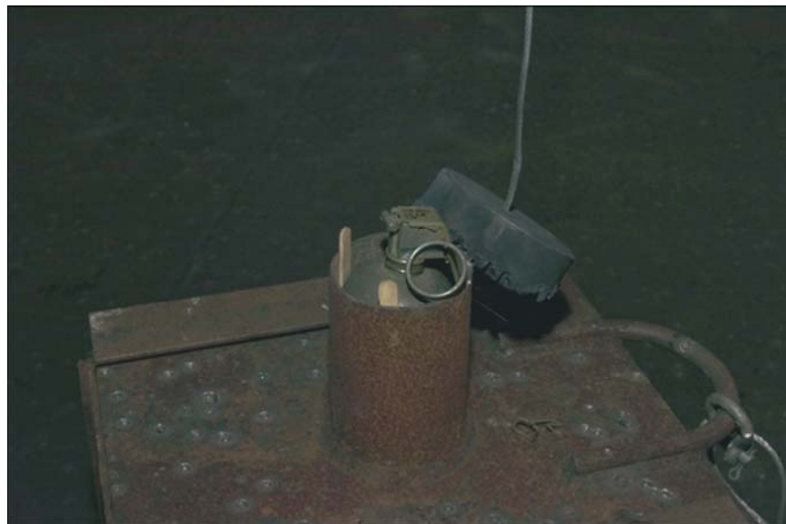
Figure 3. Grenade in cup inside LOTC.
