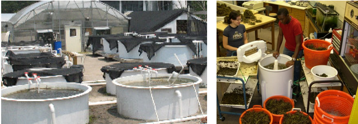
Figure 9. Seed processing equipment; large-scale outdoor seed processing tanks for Z. marina (left, photo by VIMS); wringer washing machine provides agitation to facilitate seed separation (right, photo by S. Ailstock).
