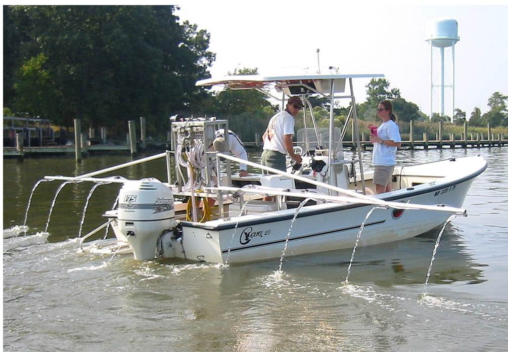
Figure 6. Mechanical seed sprayer used for eelgrass seed dispersal (photo by MDDNR).
