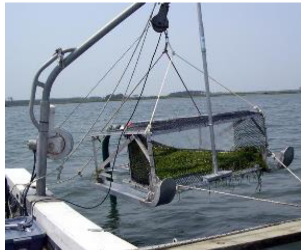
Figure 4. Portable boat-mounted aquatic reproductive shoot harvester designed by VIMS scientists (photo by VIMS).
