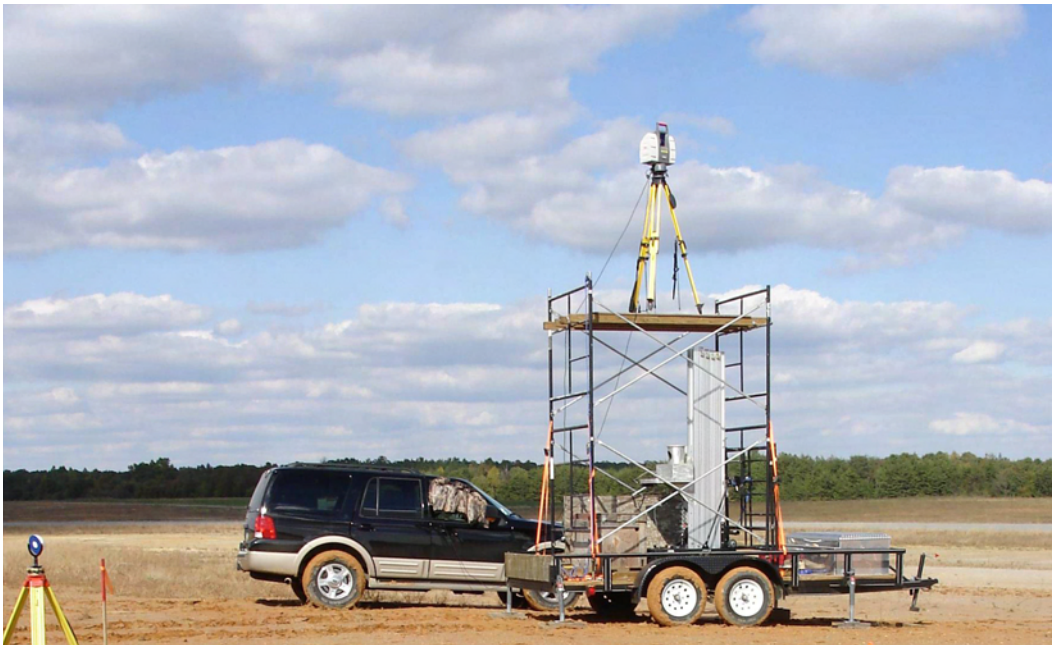
Figure 8. Trailer-mounted setup of Leica 3D laser scanner plywood scaffolding boom system.
