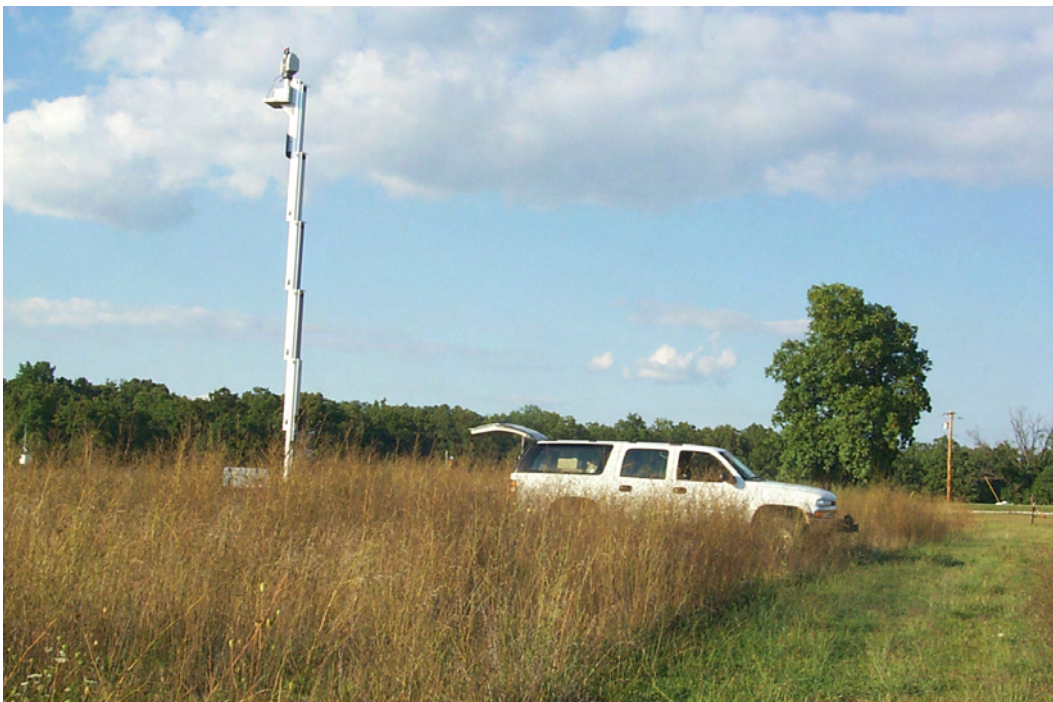
Figure 7. Trailer-mounted setup of Leica 3D laser scanner at Temperate Site D.
