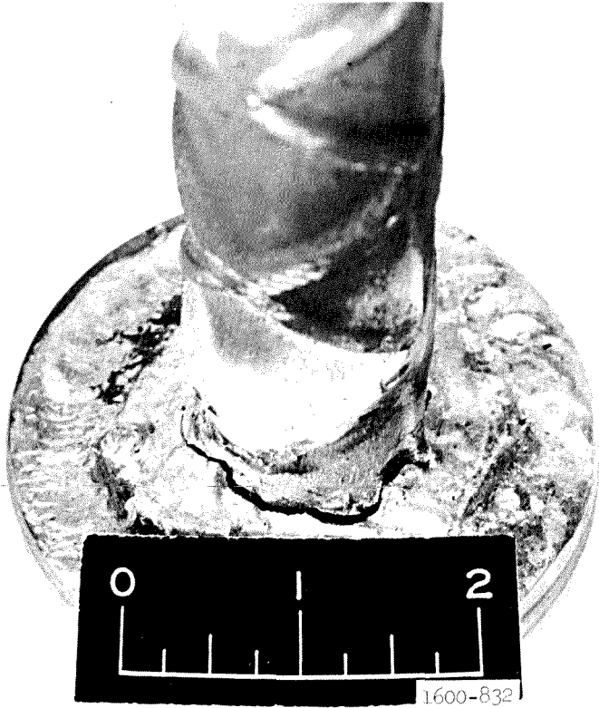
Figure 3.14 Cracked alloy-brazed joint, Test 221.
