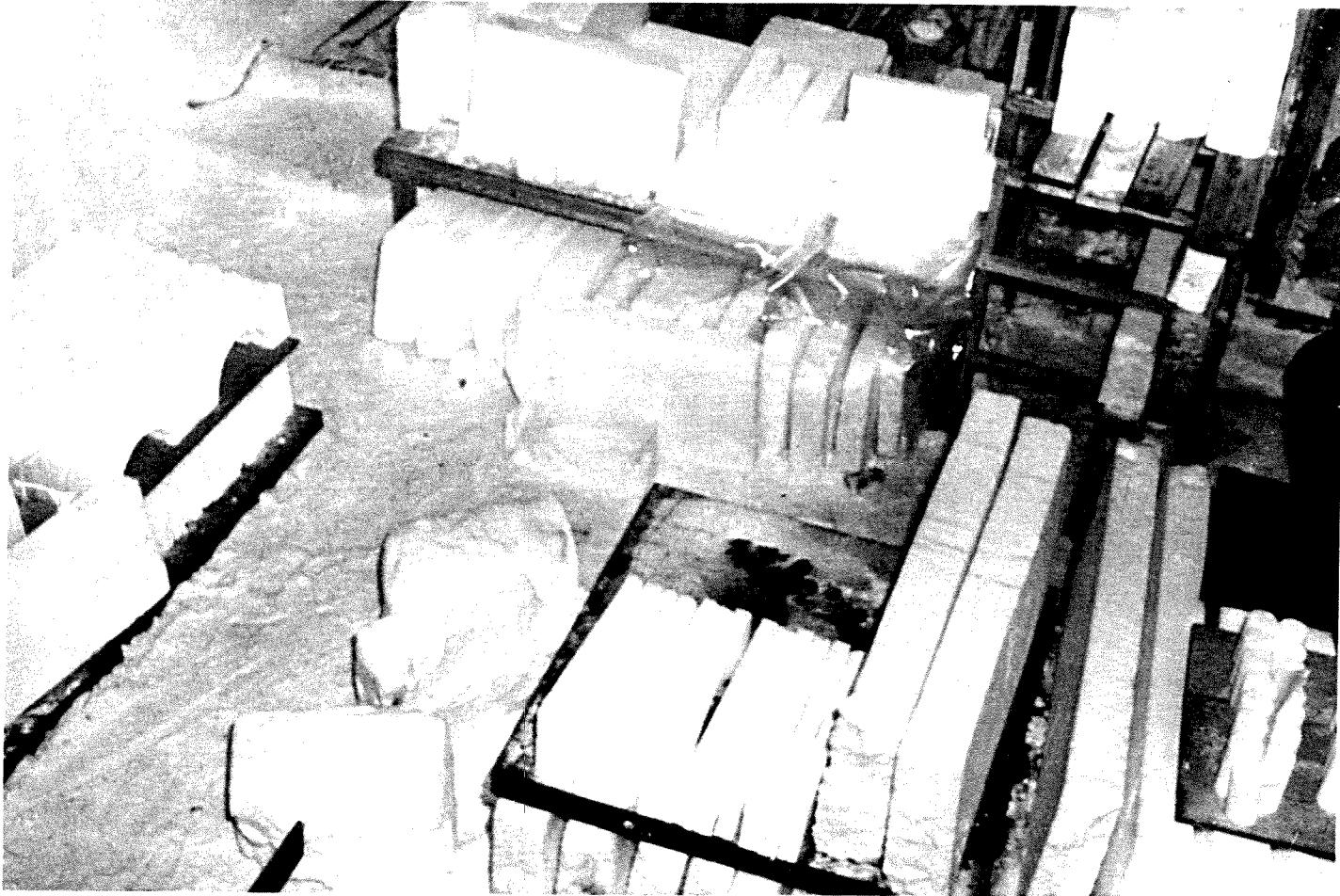
Figure 2.21 Specimen curing area and cut specimens.
