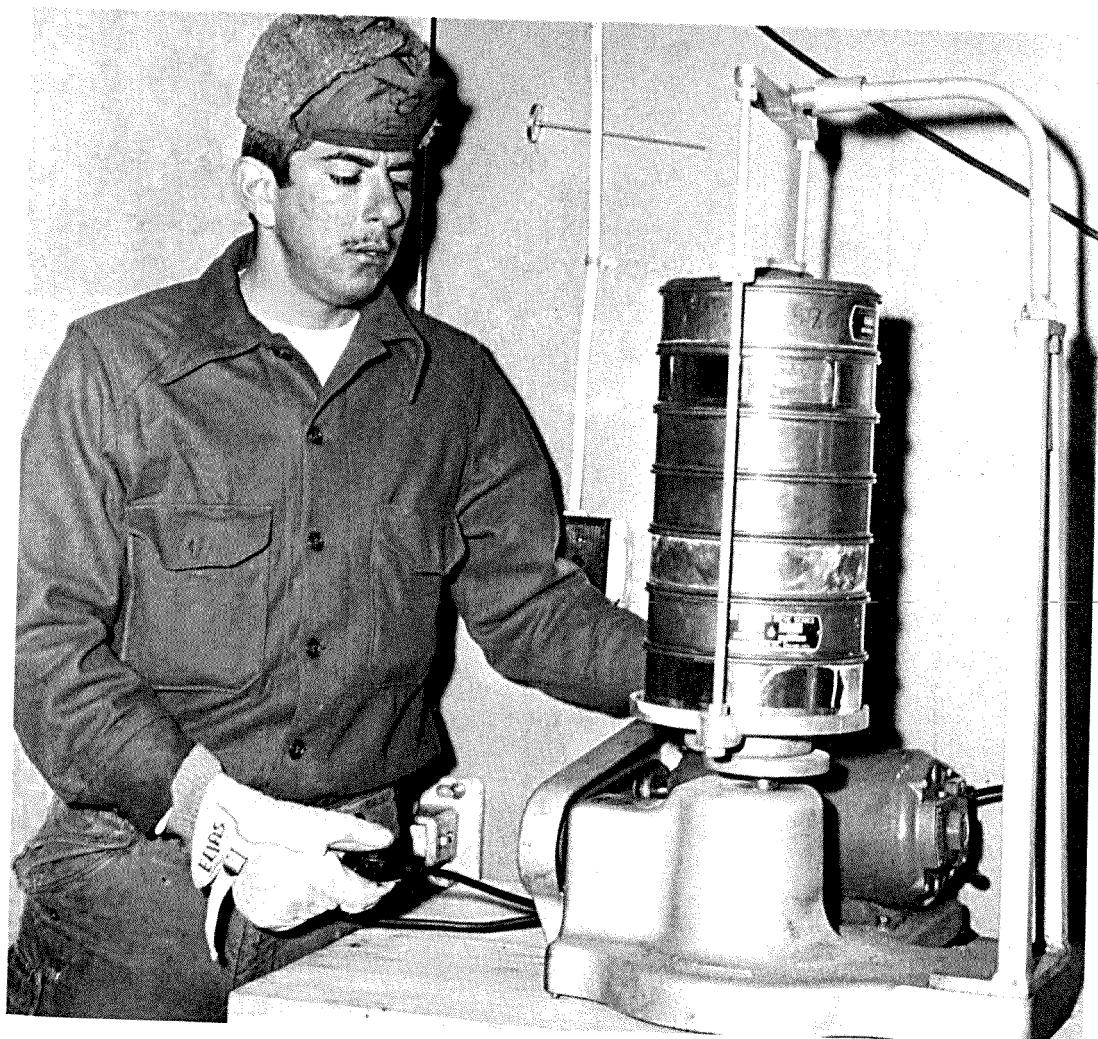
Figure 2.11 Standard sieve shaker.
