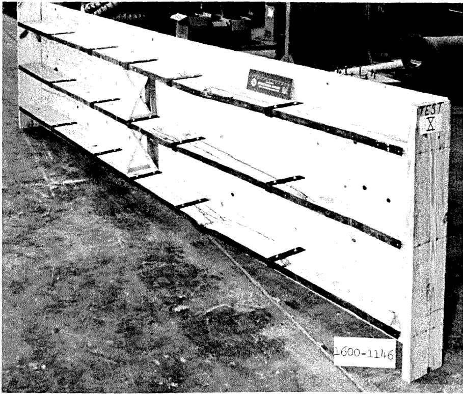
a. Overall view (note that all three joists failed).
