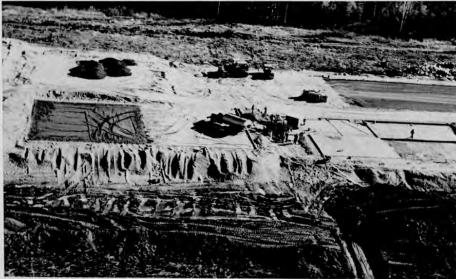
Fig. 2-40 PERMAFROST RESEARCH AREA NEAR FAIRBANKS-TYPICAL RUNWAY SECTIONS
