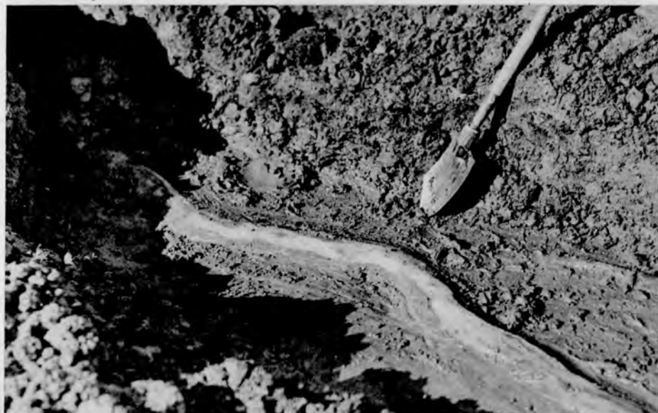
Fig. 2-14 ICE-FROZEN SOIL RELATIONSHIPS AS FOUND IN THE UMIAT POLYGON TEST SITE
