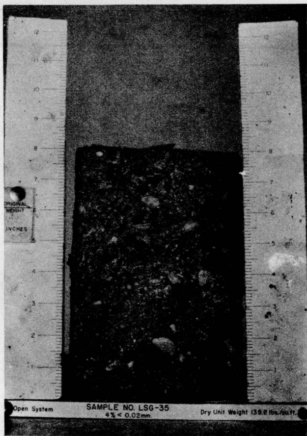
FIG. 1. LIMESTONE SANDY GRAVEL (-3/4") TEST FOR EFFECT OF RATE OF PENETRATION OF 32° F TEMPERATURE.
