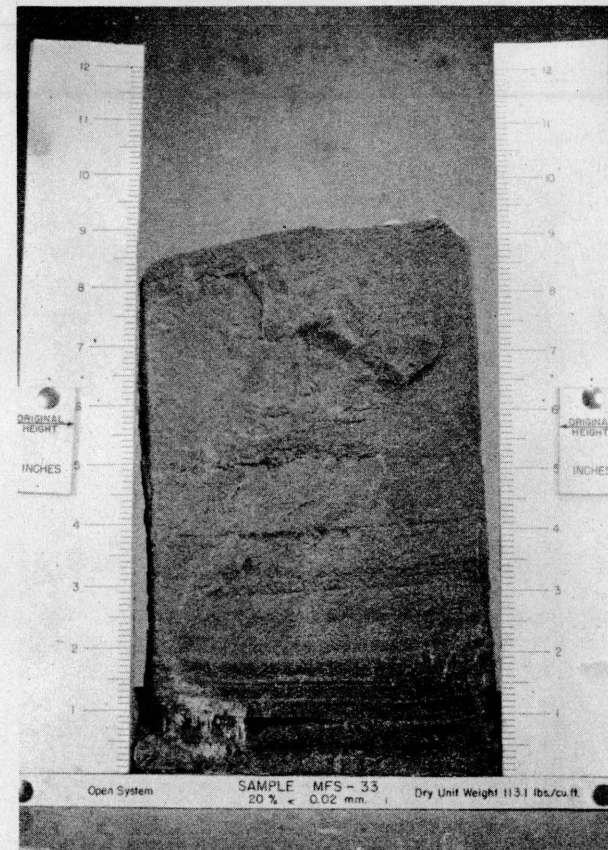
FIG. 2. MANCHESTER FINE SAND (+ #150) BLENDED WITH NEW HAMPSHIRE SILT. TEST FOR EFFECT OF PER CENT FINER THAN 0.02 MM.
