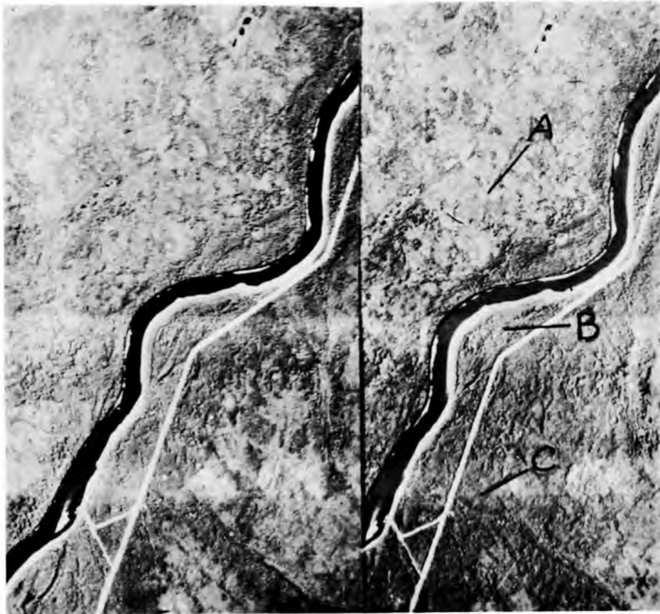
Fig. 121. Stereopair of a typical mixed forest along the Grimshaw Highway. The cover type is aspen with an admixture of white spruce and jack pine. Where aspen is the dominant tree (C), the photo texture is relatively smooth and uniform. The open stand (B) is about one-half spruce and one-half aspen. The stippled pattern on the left side of the road between B and C is produced by a stand composed principally of white spruce with a few jack pine and aspen. The sandy soil is fairly well drained under the forested areas and very poorly drained in the peat-filled bogs (A). Permafrost is found at an average depth of 2 ft in the depressions, and is absent or at depth of 5 ft or more beneath the mixed forest.
