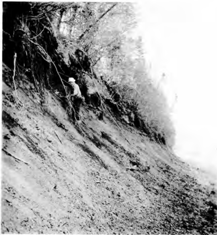
Fig. 82. Stratified silts and sands overlain by 2 ft of peat. Permafrost is exposed under peat overhang. On the surface frost was encountered in peat at 10 to 14 in. or at 14 to 36 in. in sandy silt. This exposure is on opposite bank of Mackenzie River from Carcajou Ridge.
