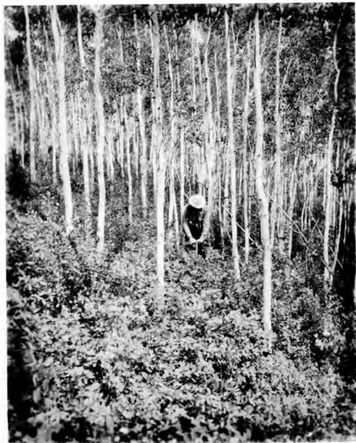
Fig. 66. Thick aspen growth on windblown silt ridge. Test pit indicated 0 to 3 in. of forest litter, 4 to 18 in. of brown powdery silt, and 18 to 36 in. of fine sandy silt. No frost was encountered in this dry, well-drained topographic position.
