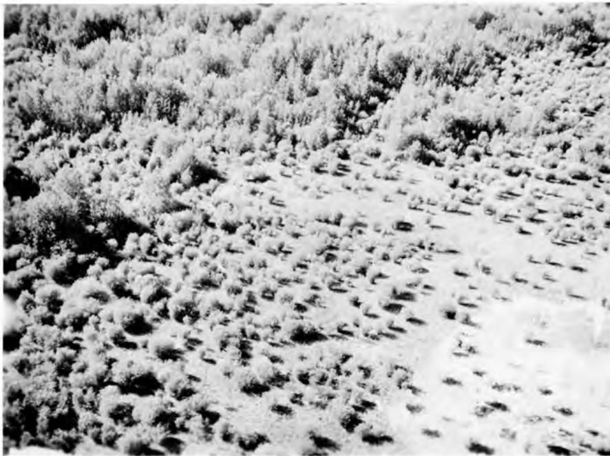
Fig. 132. A low oblique airphoto of globular willow clumps on wet fine-grained alluvium near Mills Lake. The open areas between clumps are covered with a dense sedge cover. Insulating moss mantle is thin or nonexistent. The trees located on better-drained sites are balsam poplar.
