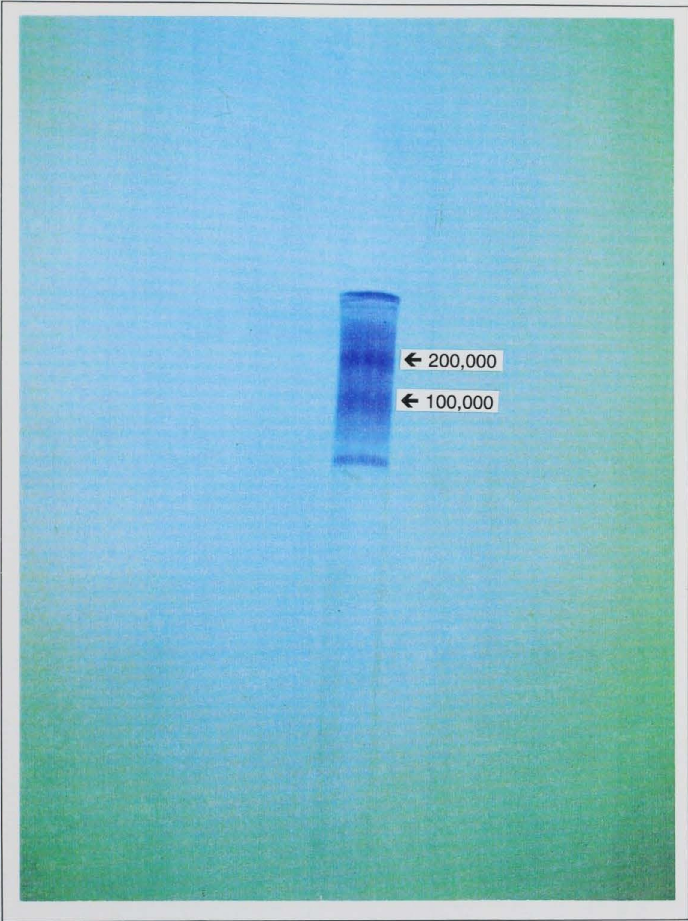
Figure 5. Polyacrylamide gel identifying a watermilfoil L-fucose-specific lectin. Two protein bands were observed in the upper portion of the gel
