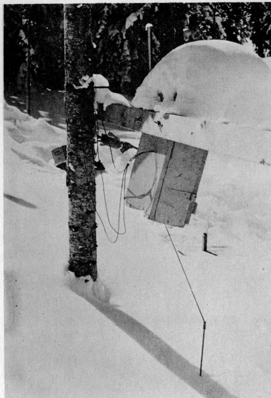
Figure 21. Settlement gage, Test field, Stevens Pass. The transmitter case is inclined for some reason and the rod, which is connected to the transmitter by a cord, is moved to the right by the creep of the snow cover. (Photograph by A. Fuchs.)
