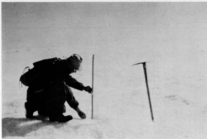
Figure 11. Typical ablation stake with taped initial level of ice at left hand. Measurement actually made vertically.
