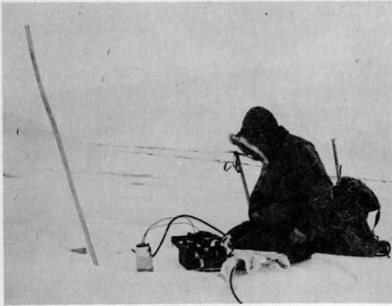
Figure 33. Measuring ice temperatures through thermocouple cable (black) with potentiometer (black box) and cold junction (vacuum bottle with wires).
