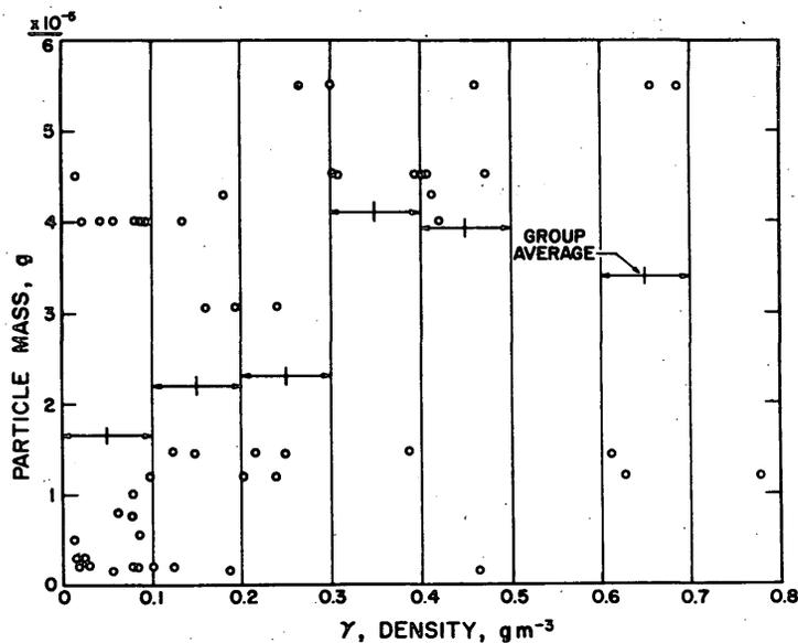
Figure 3. Mean mass of single snow particles plotted against snow density.
