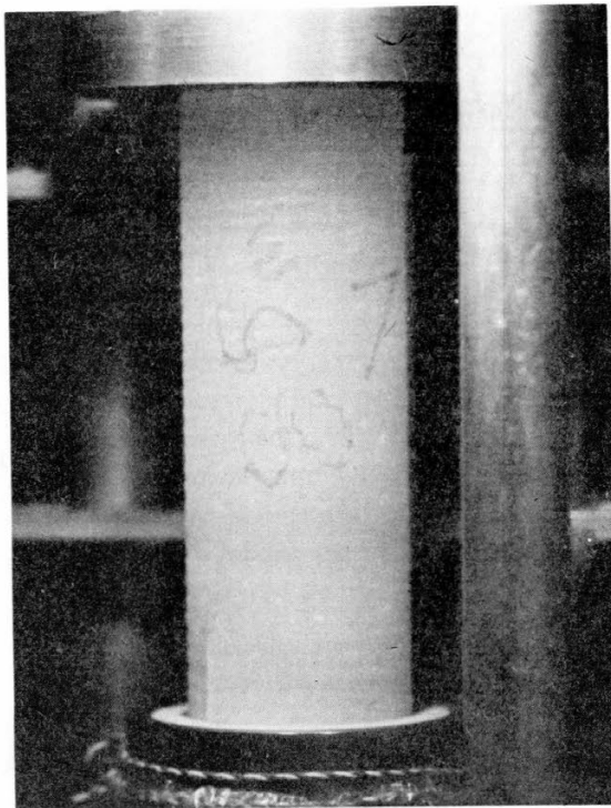
Figure 6. Crack initiation prior to failure.
