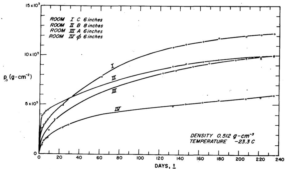
Figure 1. Plate pressure as a function of time.
