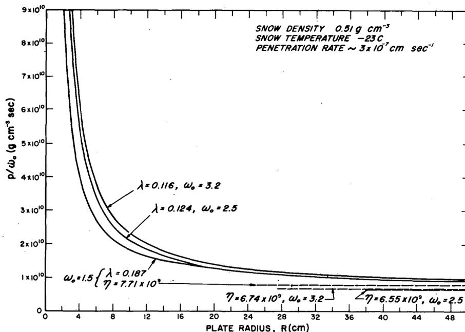
Figure 7. Effect of plate size on penetration rate and penetration resistance.
