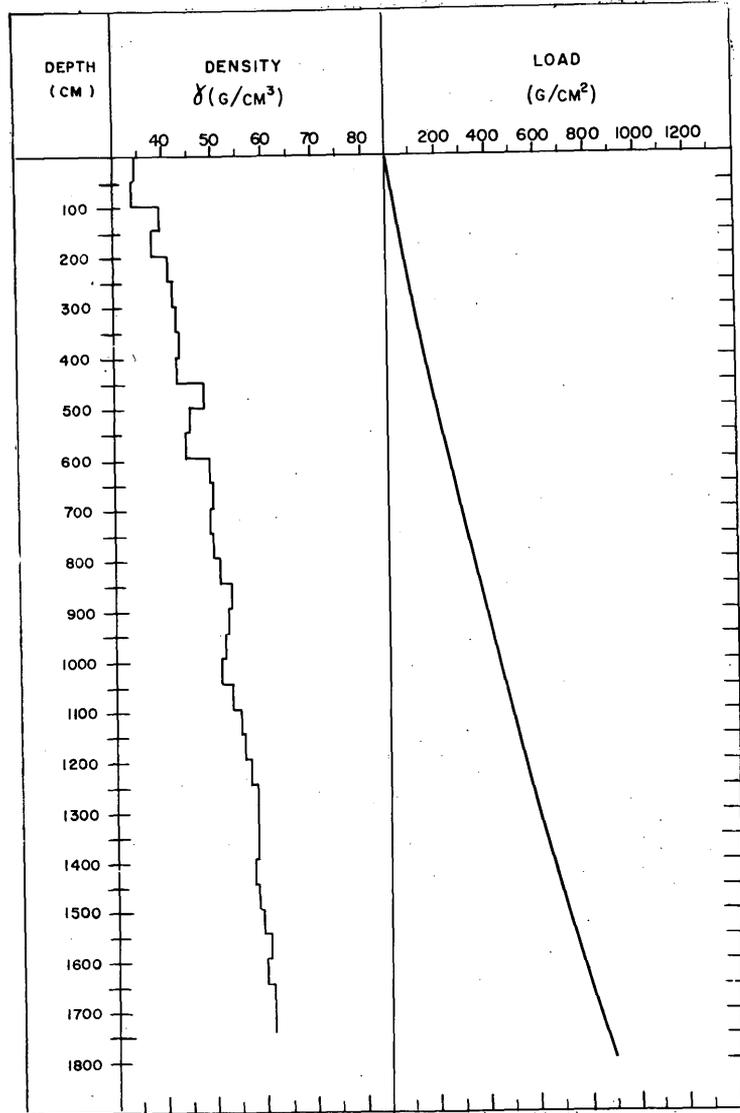
Figure 3. Snow density and overburden load plotted against depth below the ice cap surface (After Waterhouse and Steeves, 1960).
