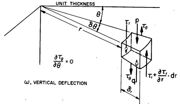
Figure 5. Stresses on an element in the shear layer.
