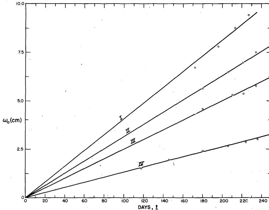
Figure 2. Plate penetration as a function of time.
