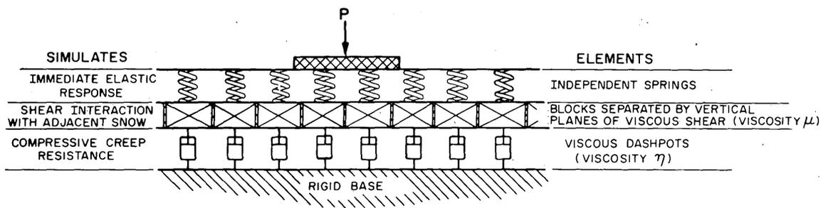
Figure 4. The Kerr viscoelastic foundation model.
