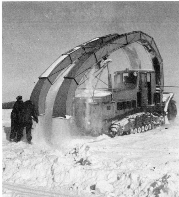
Figure 2. Peter snow plow with backcasting chutes.
