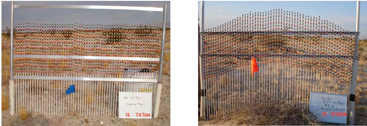
c. Surface undulation using the profilometer on level areas (left) and mounds (right). The rods are spaced 2 cm apart and each rod is vertically marked at 1-cm intervals.
