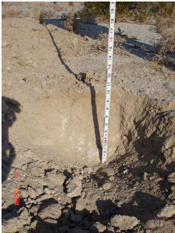
a. Cemented layer encountered showing soil clods.
