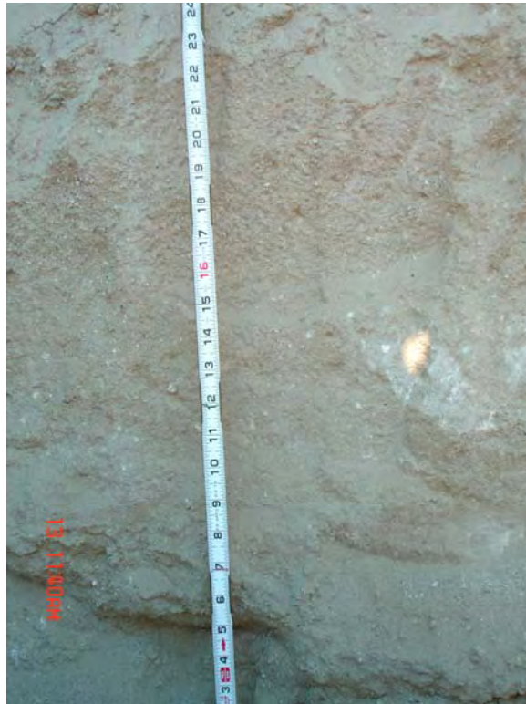
a. Pit at 9+80 2N was dug down to 0.81-m (32-in.) depth.
