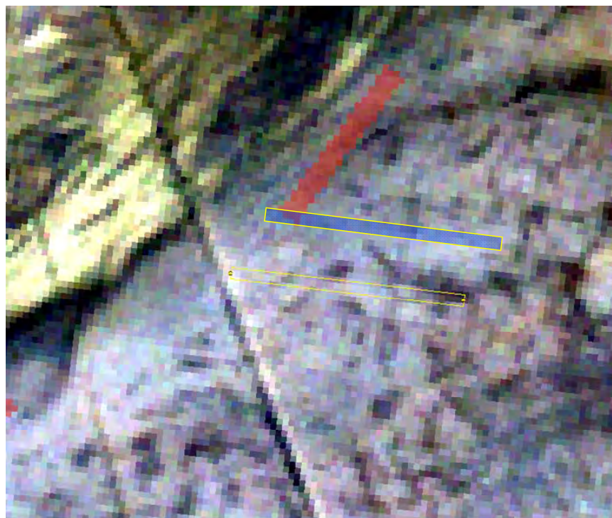
Figure 65. 1 November 2005 Landsat USGS Precision georeferenced image with Version 10 of the OLS software. Blue and red OLSs are in Precision georeferenced positions. The unfilled yellow outline OLS is the RAS field site from the Systematic georeferenced 9 May 2005 image. Filled yellow outline OLS is the field site as it should have been located from the Precision georeferenced 9 May 2005 image.
