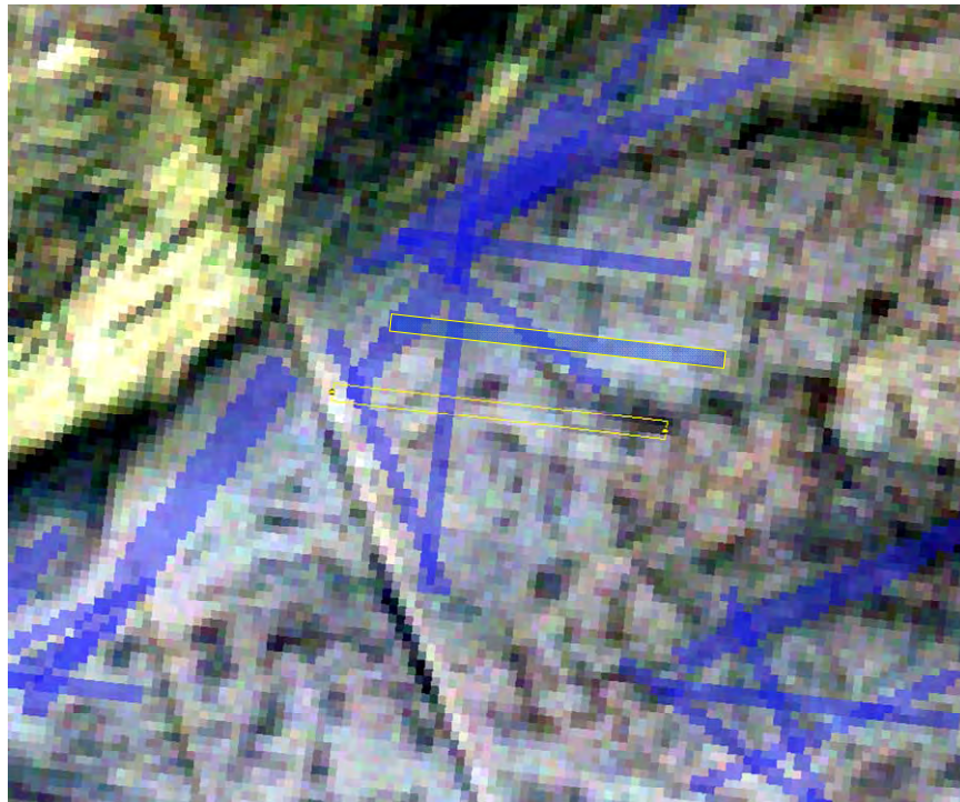
Figure 63. 1 November 2005 USGS Precision georeferenced image with Version 7 OLS software. Blue OLSs are in Precision georeferenced positions. Unfilled yellow outline OLS is the RAS from the Systematic georeferenced 9 May 2005. Filled yellow outline OLS is the field site as it should have been located from the Precision georeferenced 9 May 2005 image.
