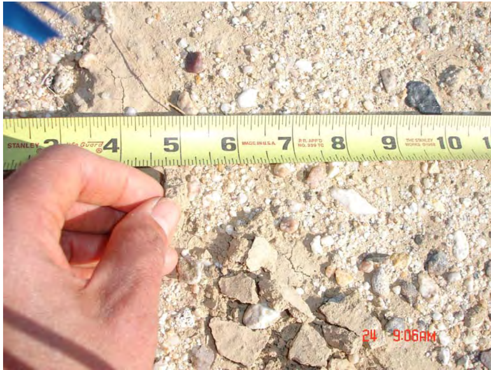
Figure 24. Cemented materials found on the surface of RAS.
