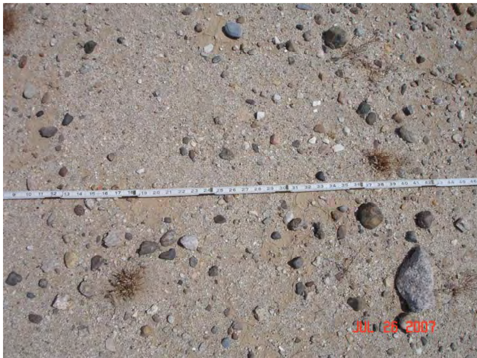
d. Stones and gravel-size materials present in sections of the RAS.
