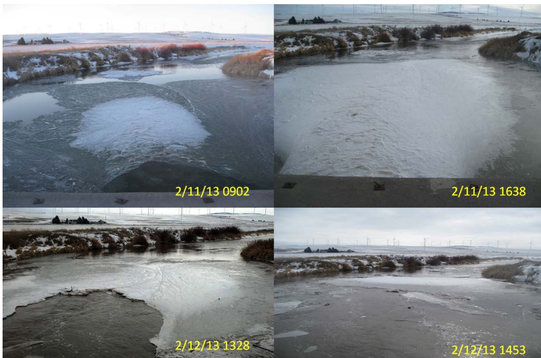
Figure 35. Evolution of the hanging ice dam immediately downstream of the Ferguson Bridge.
